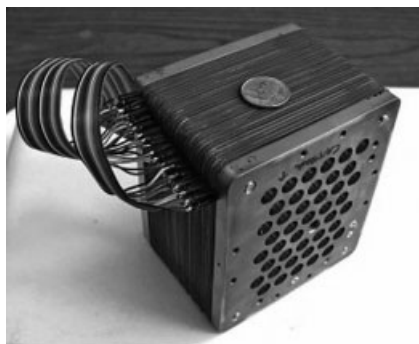
Figure 2.2 A photograph of the 30-cell DMFC stack shown together with a US Quarter for comparison of dimensions. More detailed stack properties and performance parameters for this current stack design are listed in Table 2.3.
