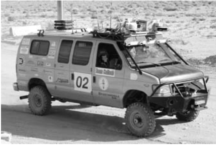
Figure 1.15: DARPA Grand Challenge. “Alice,” Team Caltech’s entry in the 2005 and 2007 competitions and its networked control architecture [54]. The feedback system fuses data from terrain sensors (cameras and laser range finders) to determine a digital elevation map. This map is used to compute the vehicle’s potential speed over the terrain, and an optimization-based path planner then commands a trajectory for the vehicle to follow. A supervisory control module performs higher-level tasks such as handling sensor and actuator failures.
