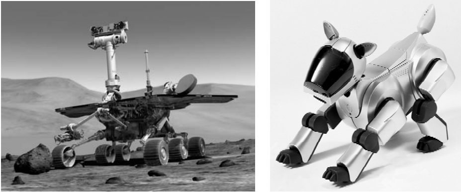
Figure 1.9: Robotic systems. (a) Spirit, one of the two Mars Exploratory Rovers that landed on Mars in January 2004. (b) The Sony AIBO Entertainment Robot, one of the first entertainment robots to be mass-marketed. Both robots make use of feedback between sensors, actuators and computation to function in unknown environments. (Photographs courtesy of Jet Propulsion Laboratory and Sony Electronics, Inc.)
