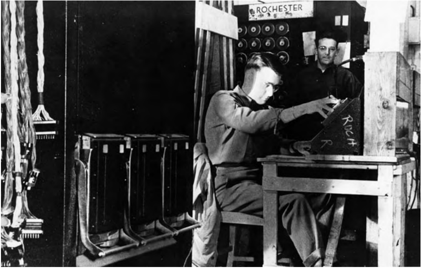
Figure 11. Working in a bombe room at Out Station Eastcote. ‘Menus’ for the outstation bombes were received from Bletchley Park over a teleprinter line.
