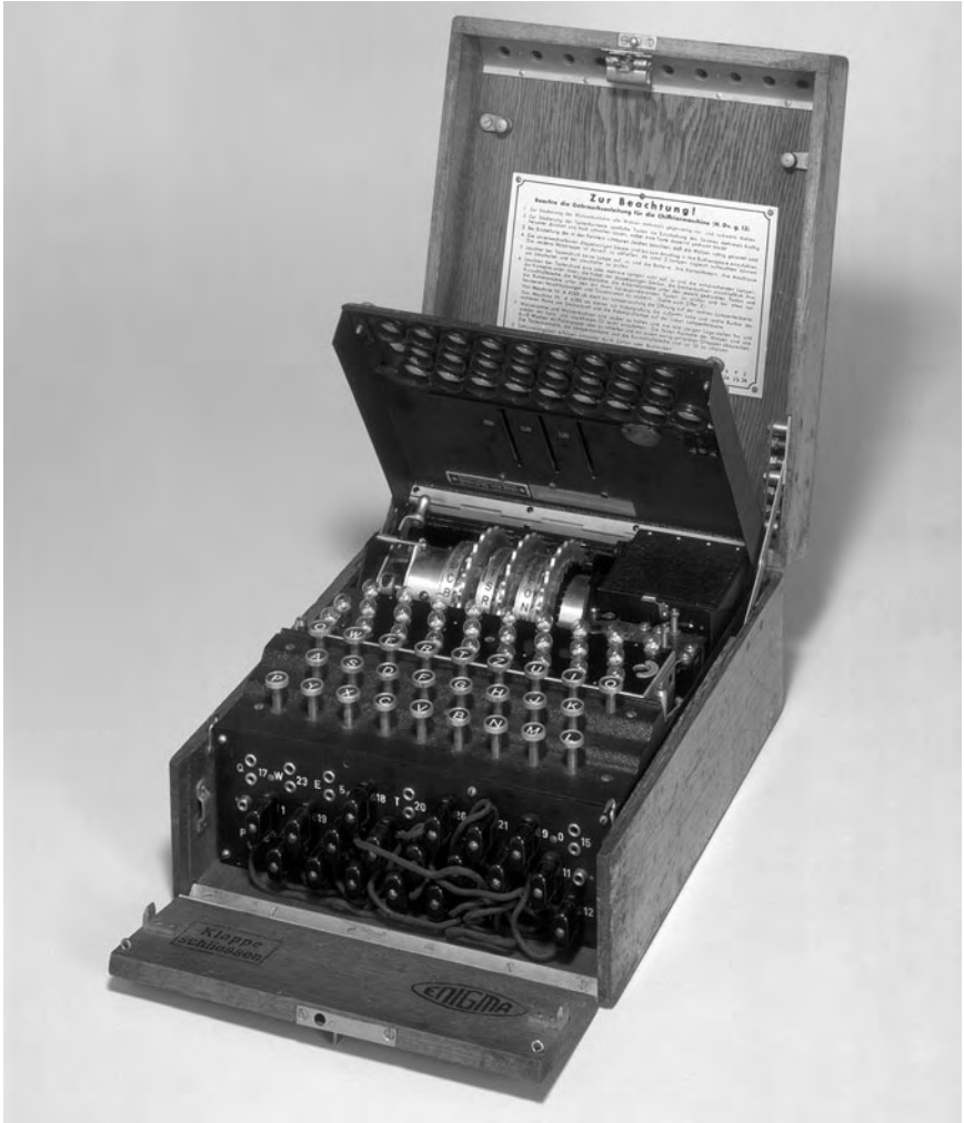
Figure 3. Enigma machine with the three wheels exposed.
