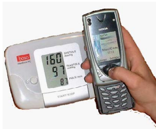
Figure 7. "MoniCam" principle: A special software application helps the user to take a photo of the display and send it to a central monitoring centre via MMS, where the values are extracted and stored in the database automatically
