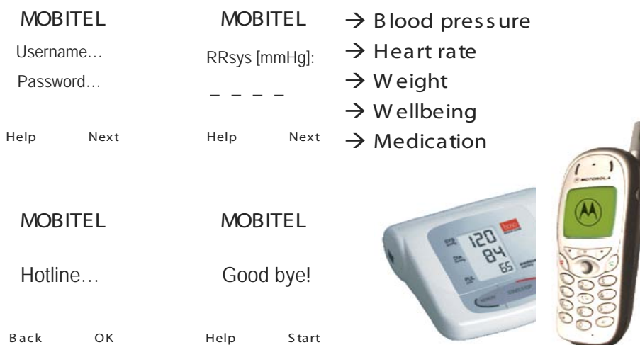
Figure 4. Graphical user interface generated by WML guides the patient through the data-acquisition process
