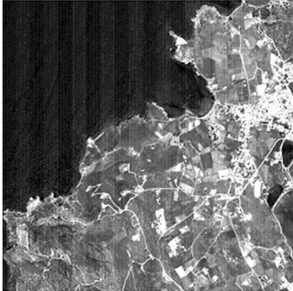
Fig. 11.13 Part of the ALOS PRISM nadir image. The noise dominates the image
