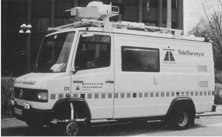
Fig. 1.2 First generation Mobile Mapping van (1990)
