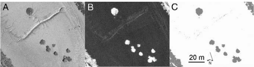
Fig. 15.2 Example of the NDVI thresholding method for mapping wetland vegetation growth after marsh restoration: (A) original imagery, (B) NDVI transform, and (C) the thresholded result; grey = vegetation and white = mud
