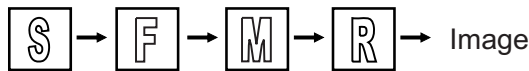
Fig. 3.5. A model of visualization that incorporates the simulation process, as well as filtering, mapping, and rendering. The simulation’s output is visualized as it is produced, so that the computation can be halted or changed according to what is seen in the results.
