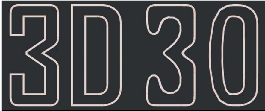
[Figure 8.3] The polygonal mesh (left) maintains the original shape, whereas the SubD mesh (right) loses its shape without proper support segments.
