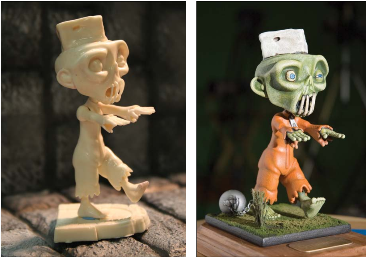
[Figure 14.15] Tofu went through several prototypes using a variety of materials. Resin was used for the figure on the left, whereas powder was used for the version on the right.
