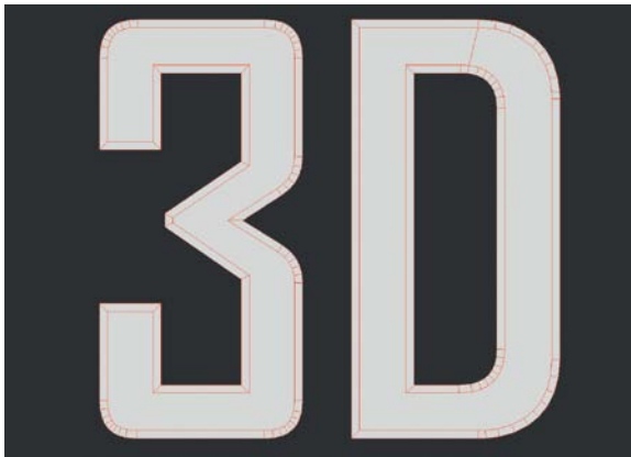
[Figure 8.2] Creating a small inset produces a clean edge loop of quad polys.
