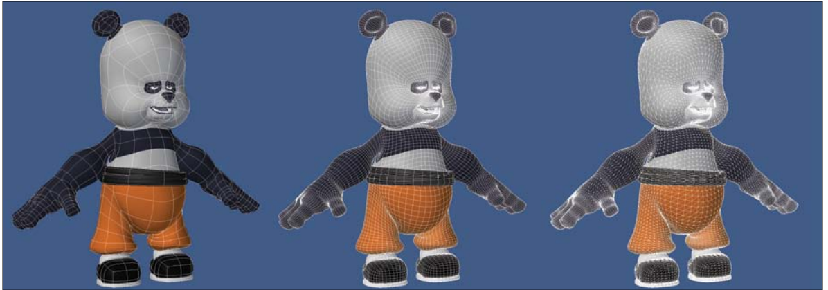
[Figure 6.2] Don't let objects created with subdivision surfaces mislead you when counting polygons. This panda character made up of 1,942 SubDs is actually 62,144 triangles at render time.
