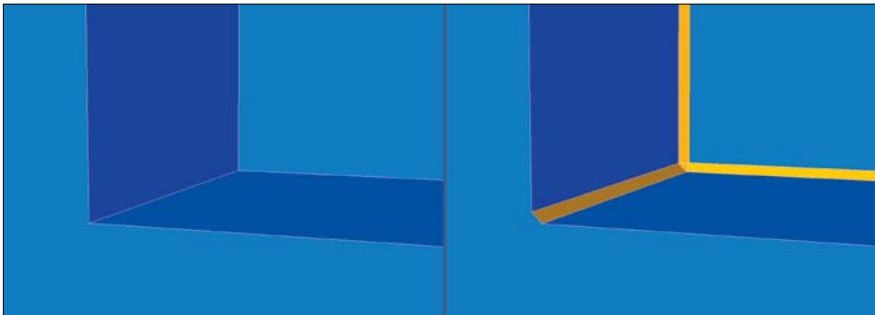
[Figure 7.11] The interior edges of this shape are also sharp and need refining (left). A fillet is applied, giving a much more realistic inner seam to this object (right).
