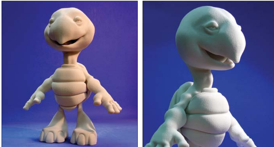
[Figure 14.8] 3D prints of digital models can be a great way to generate physical maquettes.
