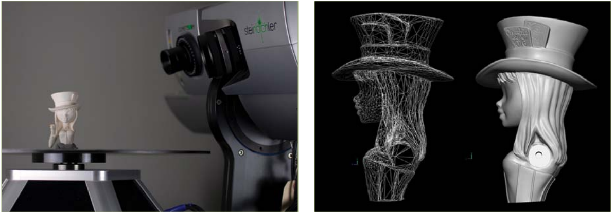
[Figure 5.12] Using a 3D scanner, Varner studios takes advantage of its 30-plus years' experience of traditional toy sculpting to create digital meshes. The physical sculpt (left) is scanned with the 3D scanner, producing a digital mesh (right).
