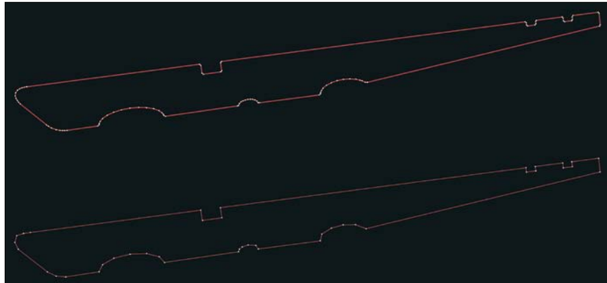
[Figure 8.13] The prong on the top uses more points to define the curves and is what I would use for a polygonal mesh. The prong on the bottom uses fewer points to take advantage of SubDs smoothing algorithm.
