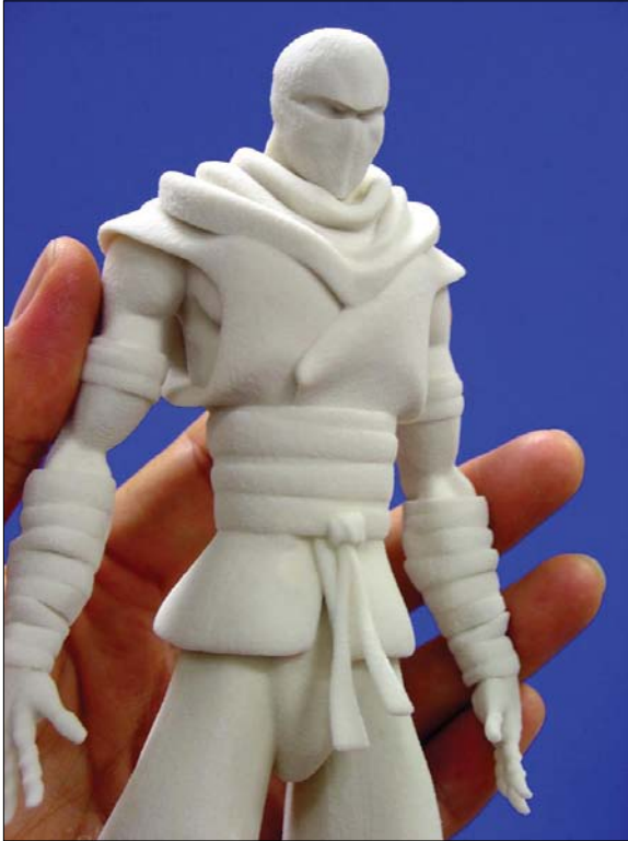
[Figure 14.11] Separate meshes can be combined during the printing process by simply having them intersect each other on your model.
