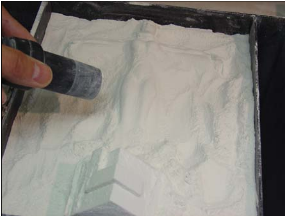
[Figure 14.5] The excess powder is removed from the chamber using a vacuum (left), and once the object is outside of the chamber, any additional powder is removed from it using compressed air (right).
