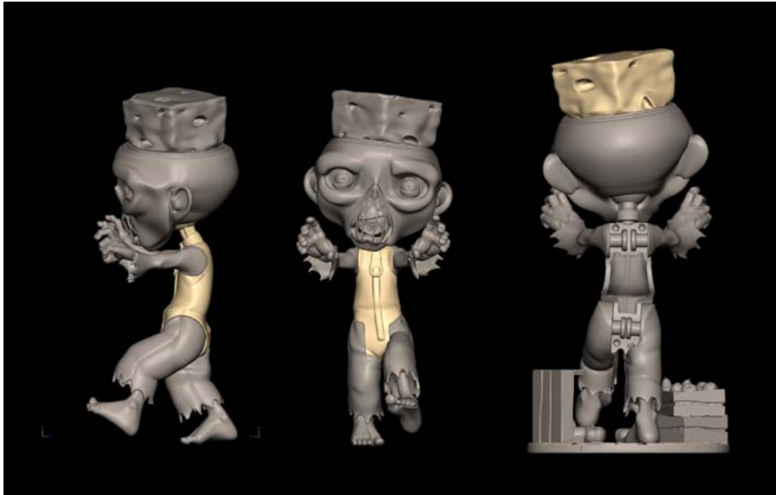
[Figure 14.17] The digital model was cut into parts for articulation (left), and the result is shown in the printed parts (right).
