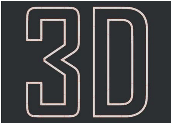
[Figure 8.5] With the support segments added in all of the required areas, the letterforms hold their shape when SubDs are applied to the mesh.
