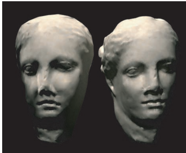
Plate XXIV. Detail transfer via normal mapping. A low resolution proxy surface (left) is rendered using the normal vector information of the corresponding high detail surface it represents.
