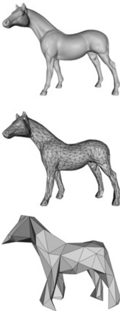
Figure 5.19. Progressive hulls as bounding volumes; a horse model with 96,966 polygons followed by its 2,000 and 200 polygon hulls.
