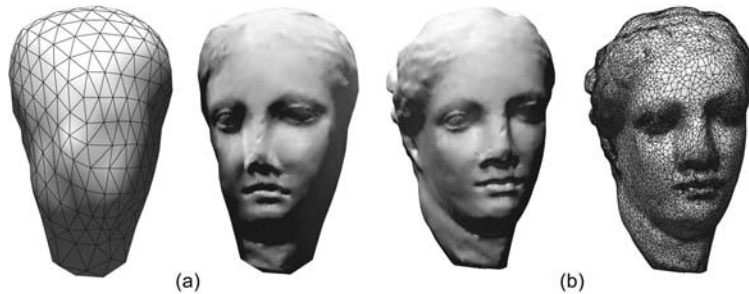
Figure 14.30. Normal mapping. (a) A low-resolution mesh has its normal vectors replaced per rendered fragment, according to the normal map of Color Plate XXII. (b) The original, high-resolution surface from which the normal map was extracted.
