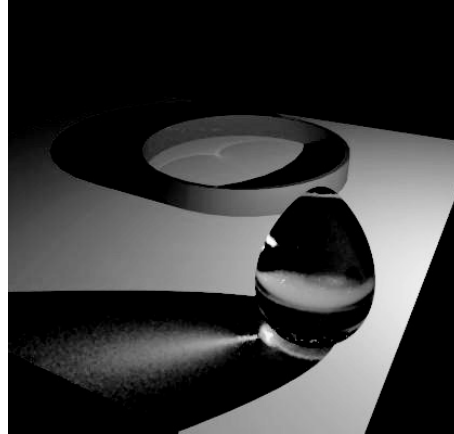
Figure 16.14. Bidirectional ray tracing. Note the extensive caustics, an effect difficult to achieve using stochastic ray tracing.
