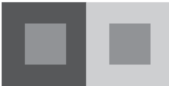
Figure 10.13. Perceived intensity levels depend on relative intensity. The inner square has the same intensity value in both images; however, on the right it appears darker (outer-region intensity on left is 50, outer-region intensity on right is 200, and inner-square intensity is 125 in both cases).
