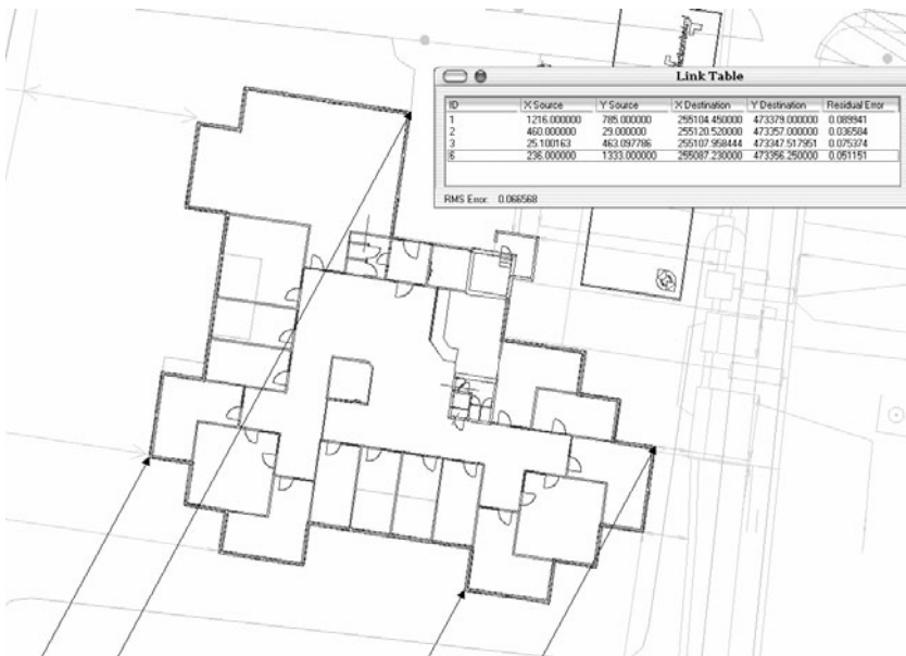
Fig. 22.2. Screenshot of the GIS used to map the APs. It shows one of the building CAD drawings (darker colours) after georeferencing on the UT overview map (light colours). The arrows show the control points, the link table depicts their un-referenced coordinates and their equivalents in RD, as well as the residual errors (all in m).
