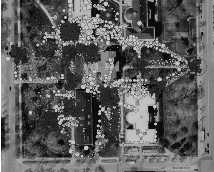
Fig. 25.6. Digital orthophoto with GPS points collected during several sections of a laboratory exercise.
