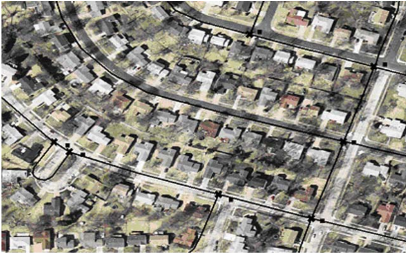
a The control point pairs detected from a road vector and imagery (The cross represents the control point in the vector, while rectangle is the corresponding control point in the image)
