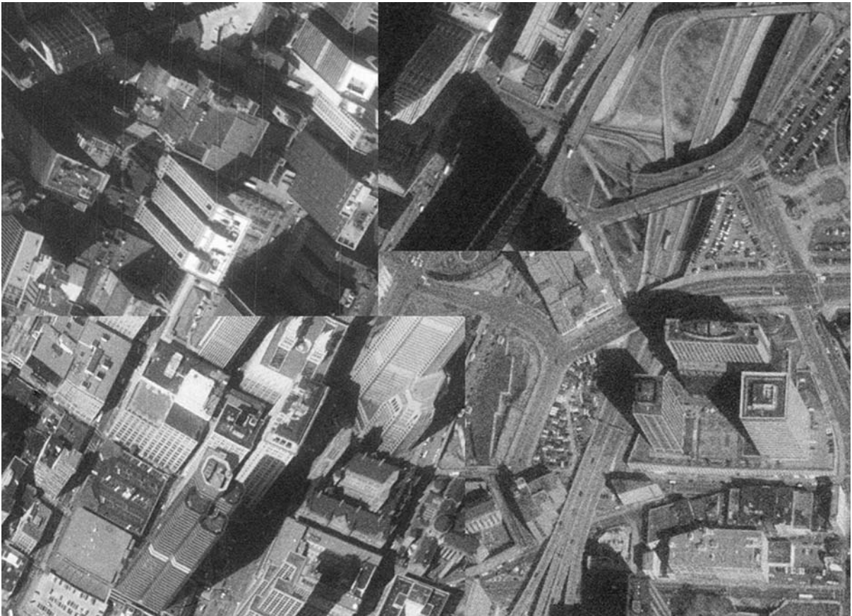
Photogrammetric Products, Figure 4 Apparent building lean in an orthomosaic, particularly evident at the mosaic seams. Notice that features at ground level are aligned
