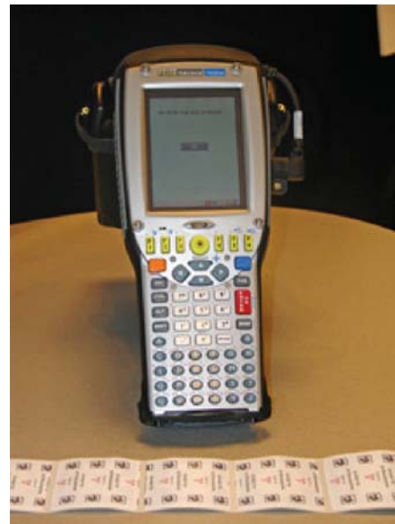
Radio Frequency Identification (RFID), Figure 4 Mobile RFID reader with tags in foreground. (Source: PM J-AIT)
