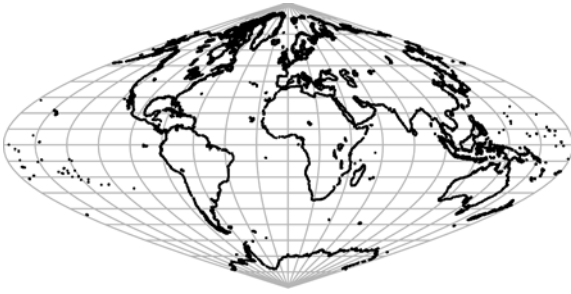
Mathematical Foundations of GIS, Figure 9 Sinusoidal projection of the world
