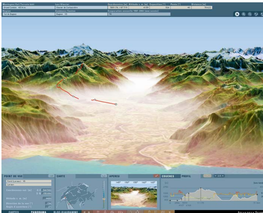
Multimedia Atlas Information Systems, Figure 2 Example of a 3D atlas: 3D display of evaporation data as overlay on a digital elevation model, combined with a satellite image and atmospheric effects. The user-defined profile shows both a topographic and thematic section ( lower right ). © Atlas of Switzerland
