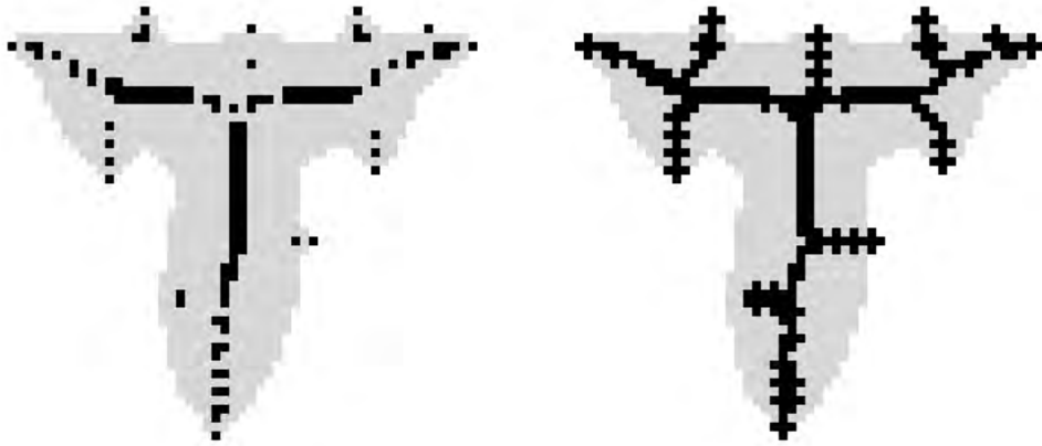
Figure 5.2.1. Disconnected and connected Pavlidis skeletons of the SR71.
