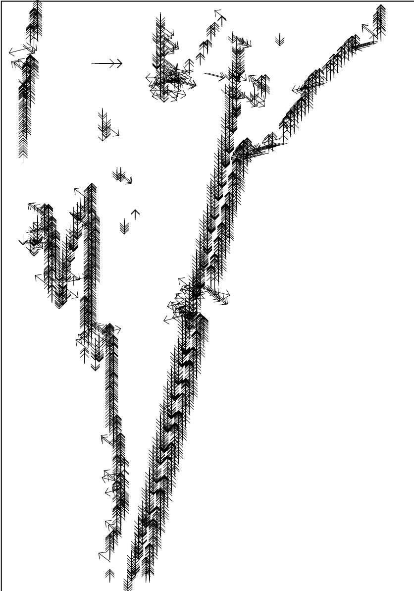
Figure 3.10.3. Edge points with their associated directions.
