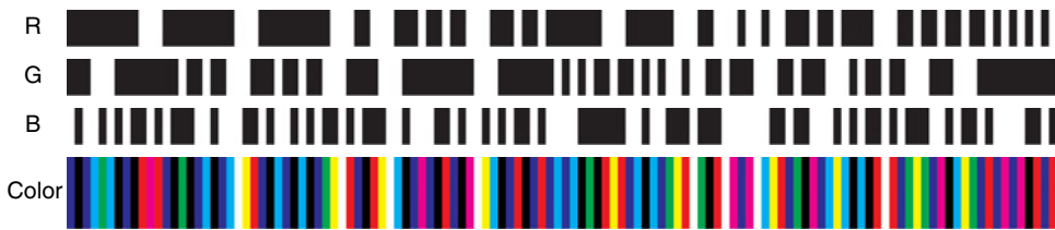
Figure 8.21. Zhang et al.'s color stripe pattern created using a de Bruijn sequence of order 3 over five symbols.
