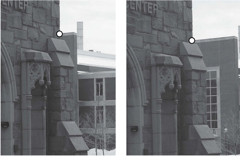
Figure 6.2. A false corner introduced by a coincidence of perspective between two surfaces: one in the foreground and one in the background. From the positions of the chimney and the corner of the background wall in the two images, we can see that the white feature points don't correspond to the same 3D location, even though the pixel neighborhoods are almost identical.
