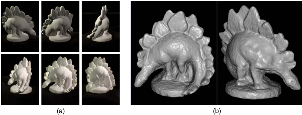
Figure 8.27. (a) Six of sixteen input images for a multi-view stereo algorithm. (b) Two views of the 3D result of PMVS (after creating a triangle mesh from the estimated points).
