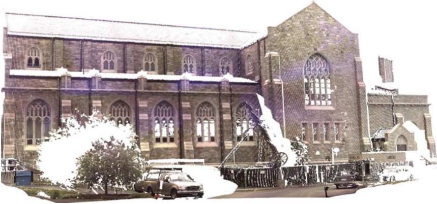
Figure 8.5. A co-registered color camera can be used to texture-map the points in a LiDAR scan, making it more understandable.
