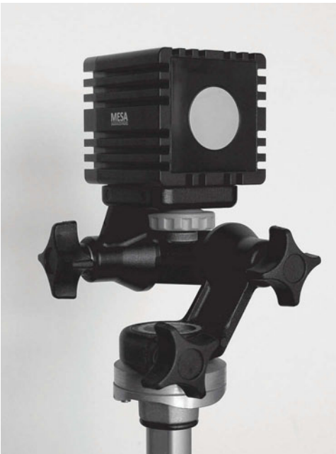
Figure 8.8. A flash LiDAR device, also known as a time-of-flight camera. The CMOS sensor in the middle (the silver circle) is surrounded by a bank of infrared LEDs that illuminate the scene.
