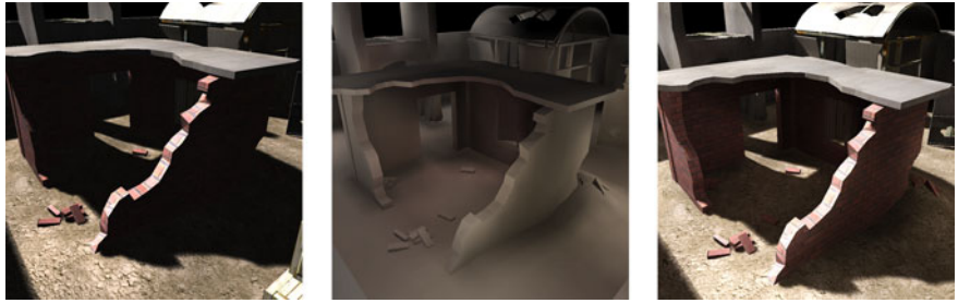
Fig. 8 From left to right: direct only lighting, indirect illumination using our method and final image with direct and indirect lighting
