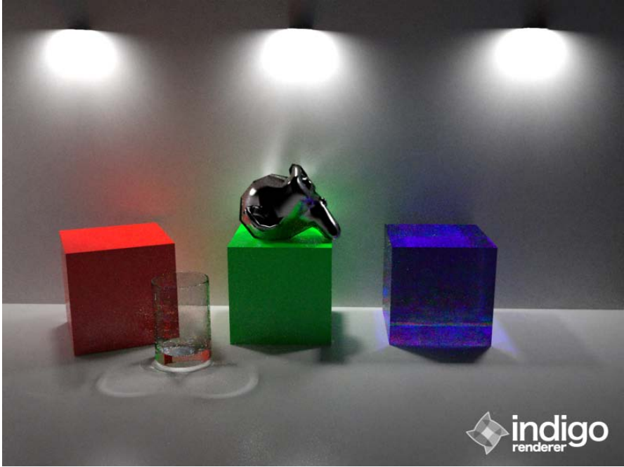
Fig. 9 Example of rendering using a standard IES (center light), MLP (right light) or ECON (left light) as approximator in the same scene. Rendering is performed using Indigo Renderer.
