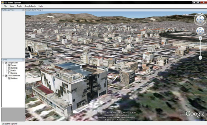
Fig. 11 Using GIS-Scene-Explorer for free navigation into georeferenced scenes containing 3D building models with texture
