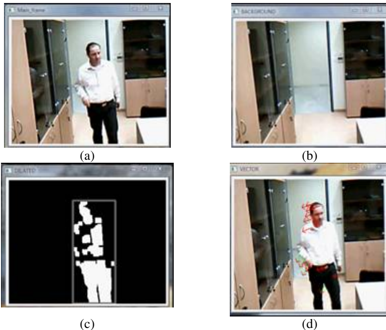
Fig. 2 Foreground isolation using the proposed methodology. (a) The original captured image frame. (b) The background content. (c) The detected foreground object. (d) The motion information of this image frame.
