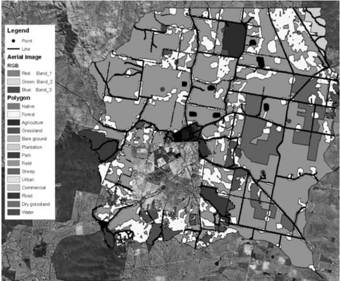
Fig. 25.3. Screen shot of NASA World Wind : the polygon feature was imported through a KML file and the screen overlay, point and imagery were added through an edited XML file
