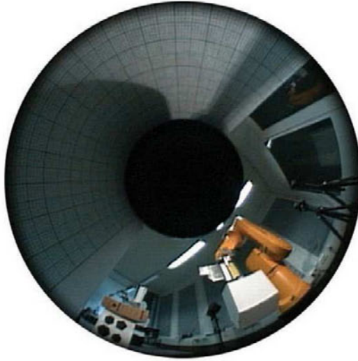
Fig. 7.1 Typical image taken with a catadioptric camera with a parabolic mirror
