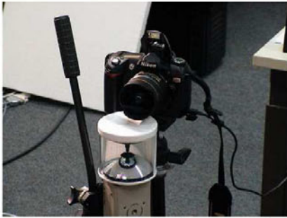
(a) Setup of a standard camera above a catadioptric camera with a parabolic mirror
