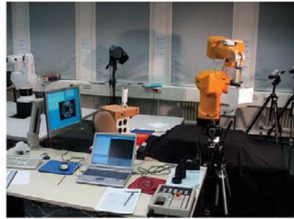
(b) Setup of cameras relative to robot arm
