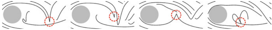
Fig. 6 Path lines in the flow behind a cylinder have been seeded using Algorithm 1, but without excluding the areas around cusp seeding lines. While the result is free of (self-)intersections, some path lines exhibit cusps or cusp-like shapes (highlighted by red circles)
