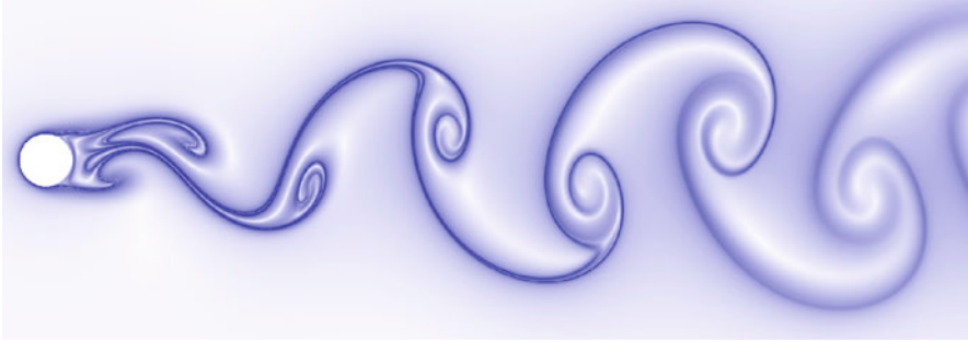
Fig. 5 L-FTLE computed for the cylinder dataset computed for two shedding periods. White color corresponds to low and blue to high FTLE values
