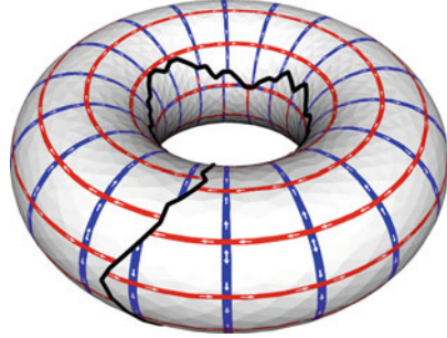
Fig. 6. Parameterization after the first stage. Grid lines are discontinuous across the cuts.
