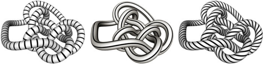
Fig. 7. Left: Only u coordinates are used to map stripes on the knot surface. Middle: Only v coordinates are used. Right: u and v coordinates are used. The texture image is a diagonal line which connects two opposite corners.
