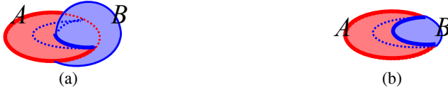
Fig. 1. Configurations of two contact relations, derived from the topological region-region relations in (a) Fig. 8U 1 and (b) Fig. 8e 1 , in which the region A is clipped by the region B
