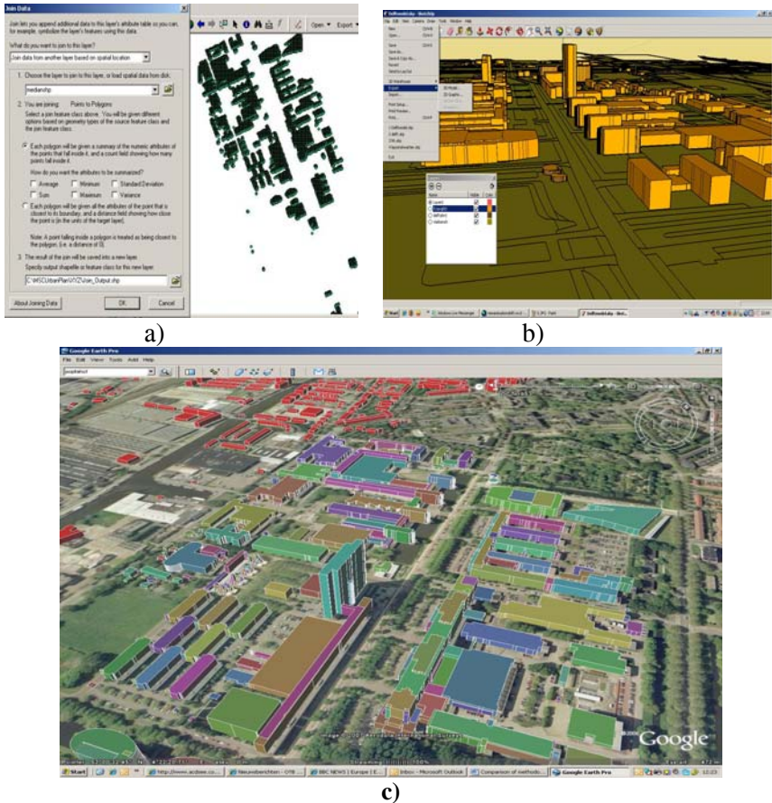
Fig. 3. Snapshots of a) filtering laser scan points in the outlines of the buildings, b) 3D reconstructed model in ArcGIS and c) 3D block model of buildings in Google Earth. (courtesy, Kibria, 2008).
