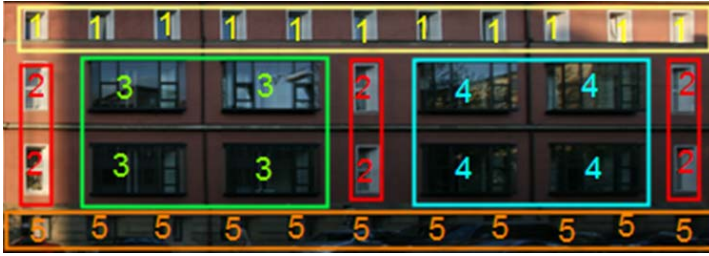
Figure 1: By observation on the rectified facade we can decide the number of layers. In this example we need 5 layers for the windows and one layer for the wall.
