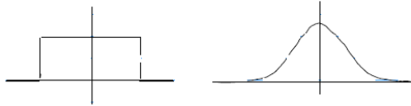
Fig. 10. a) a pillbox function describing a camera sensor b) the Gaussian with a variance \sigma
