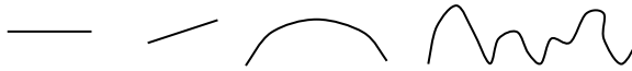
Figure 2.2 Relationship between curvatures and complexity: the curvatures of the left two lines are 0 as the radius is infinite while the line on the right side has large curvatures as the radiuses are small.
