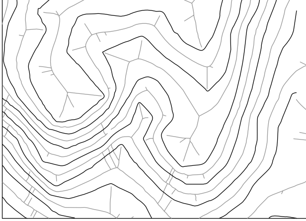
Figure 5.25 Contour map with extracted skeleton lines (Thibault and Gold 2000).
