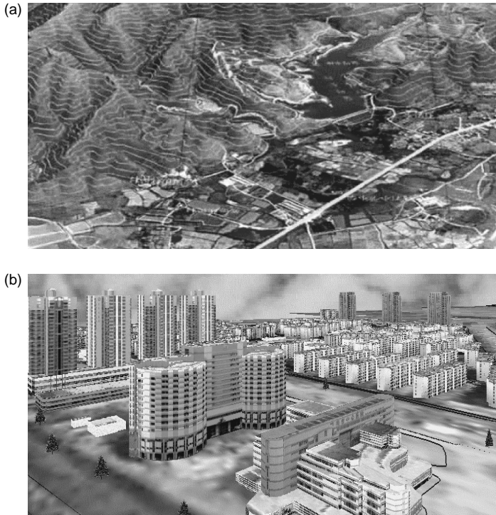
Figure 12.18 Virtual landscape by mapping texture and other objects: (a) texture image and 2-D features mapped onto DTM and (b) texture image and 3-D features mapped onto DTM. The color plate can be viewed at http://www.crcpress.com/e_products/downloads/download.asp?cat_no=TF1732 .
