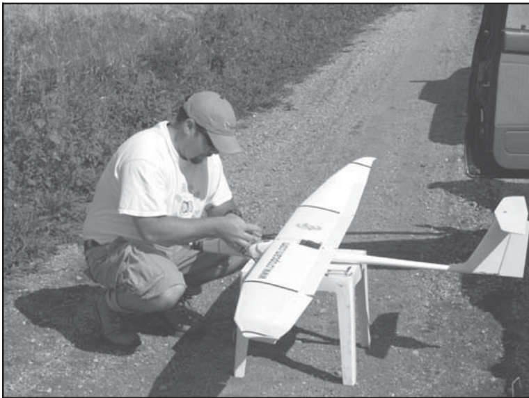
Fig. 1 Setting up the CropCam UAV in the field
