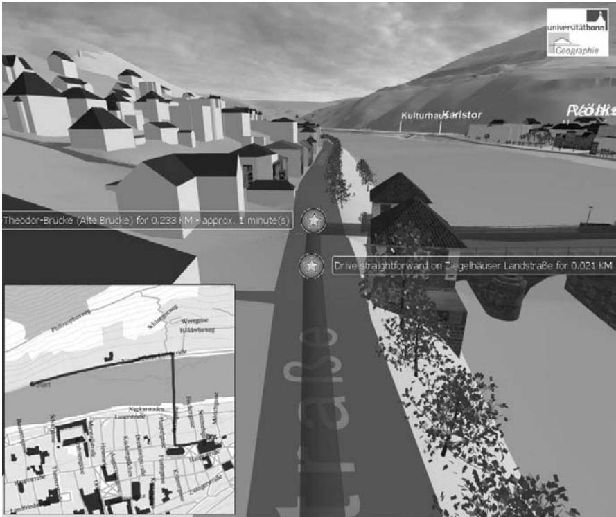
Fig. 8.9. Display of a route integrated into a 3D city model with corrected road surface. The route goes right onto the bridge.
