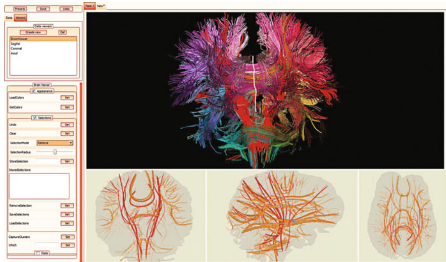
Fig. 5 An interactive analysis system using linked views and planar tract-bundle projections. Three planar representations, along the coronal, transverse and sagittal planes ( bottom panels ), are linked to a 3D streamtube model ( upper left ) and a 2D point embedding of tract similarities ( upper right ). Selections in the projection views can be made by clicking or cutting across cluster curves and are mirrored in the 3D view. Points corresponding to the selected tracts are interactively embedded into the plane and used to refine selections at the tract level
