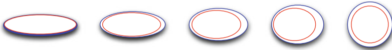
Fig. 1 Determinant Versus Trace. All blue tensors have the same trace while all red tensors have the same determinant as the tensor on the left . Tensors with a preserved trace have a higher volume (swollen) than those with a preserved determinant
