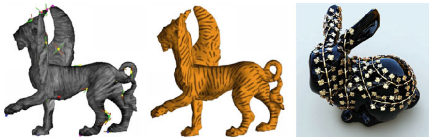
Fig. 1 A vector field is needed to guide texture and geometry synthesis on surfaces. The singularities in the vector field ( left ) can lead to the breakup of the synthesis pattern ( middle ). A leaf pattern is placed on the Bunny surface following a vector field (not shown) (The right image is a courtesy of [23], ©2011 IEEE)
