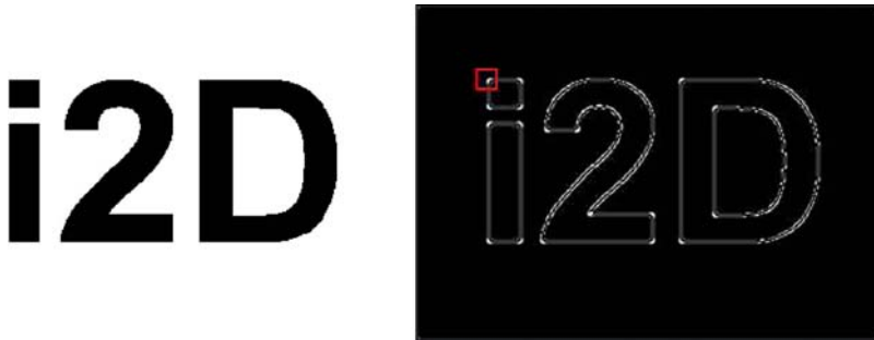
Fig. 4. Original image and local information by the determinant of the even part of the monogenic curvature tensor. One representative i2D corner is marked by the small rectangle
