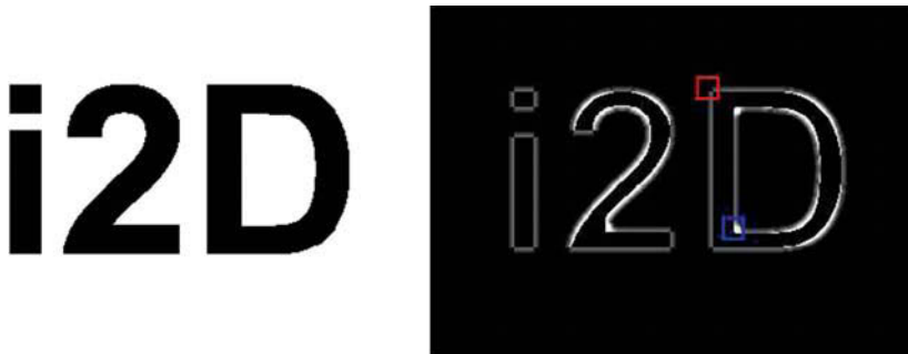
Fig. 5. Original image and local angle of intersection information. The monogenic curvature tensor is able to differ between inner and outer corners. Both the black corner with intersection angle of 270^\circ as well as the white corner with intersection angle of 90^\circ are marked by a rectangle
