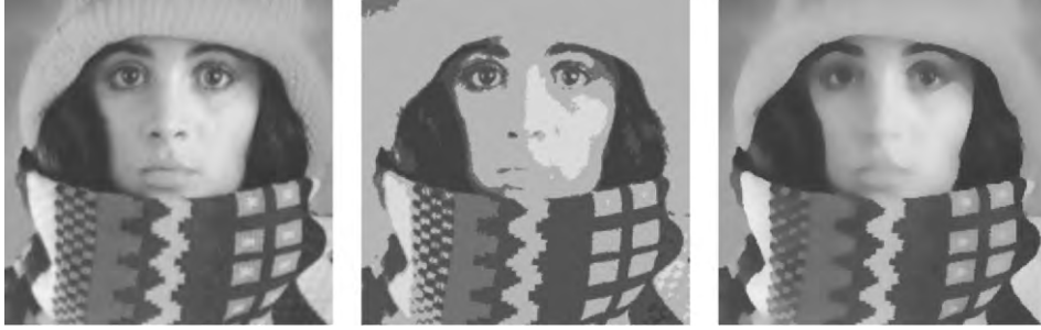
Figure 18.2. Local mode filtering. (a) Left : input image. (b) Center : iteratively smoothed using eq. (5) and the penaliser from Table 18.1(c) in a global spatial window. This approximates mode filtering of the histogram. (c) Right : processed with the local iterative filter from eq. (9). The tonal weight g(s^2) = \exp(-s^2/\lambda^2) was combined with the soft spatial window (8) with \theta = 5 . This approximates a local mode filter.
