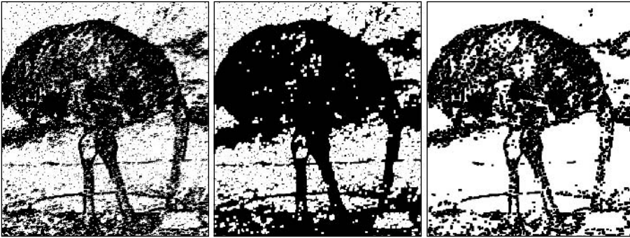
FIGURE 15.7 Left: noisy binary picture P ; note that black pixels have value 1. Center: result of closing P using N_8 . Right: result of opening P using N_8 .
