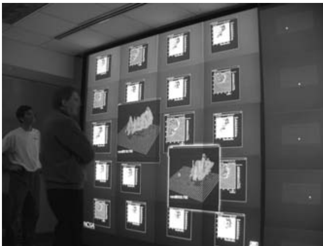
Figure 44.18 Tiled wall display of ensemble WRF model simulation. Image courtesy NCSA. (See also color insert.)
