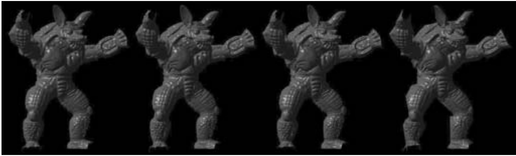
Figure 20.2 Four discrete LODs of the armadillo model (2 million triangles) using normal maps [15]. LODs have 250,000, 63,000, 8,000, and 1,000 triangles, respectively. Copyright © 1998 Association for Computing Machinery, Inc. (See also color insert.)
