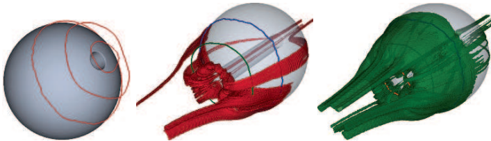
Fig. 2. Left image: Vortex cores lines of used dataset (according to the method of Sujudi-Haimes [14]) after a filtering step. There are three main ring vortices. Middle and right picture: Characteristic sets A_{v1} and A_{v2}
