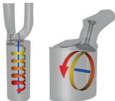
Fig. 3. (left) The swirl motion of flow in the combustion chamber of a diesel engine. Swirl is used to describe circulation about the axis aligned with the valve cylinder. The intake ports at the top provide the tangential component of the flow necessary for swirl. The data set consists of 776,000 unstructured, adaptive resolution grid cells. (right) Some in-cylinder flows require a tumble motion flow pattern in order to mix fuel with oxygen. Tumble flow circulates around an axis perpendicular to the cylinder axis, orthogonal to the case of swirl motion
