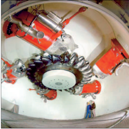
Fig. 2 (p. 28). Pelton turbine with five injectors.
