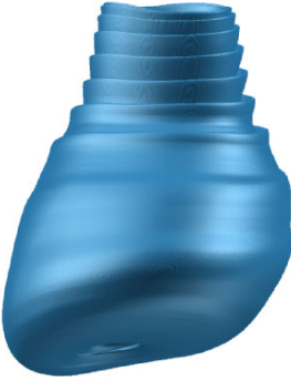
Fig. 13. Isosurface of the voxel-sampled single streamline on the surface of the breakdown bubble.
