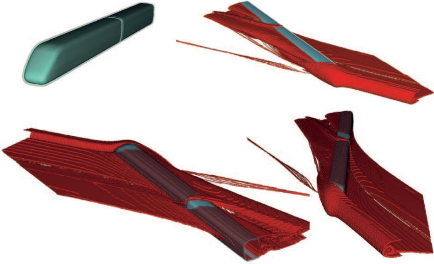
Fig. 1. Boundary of the characteristic set A of the flow structure \mathcal{G}_{Surface} . (Upper left picture shows the hull around the train.)
