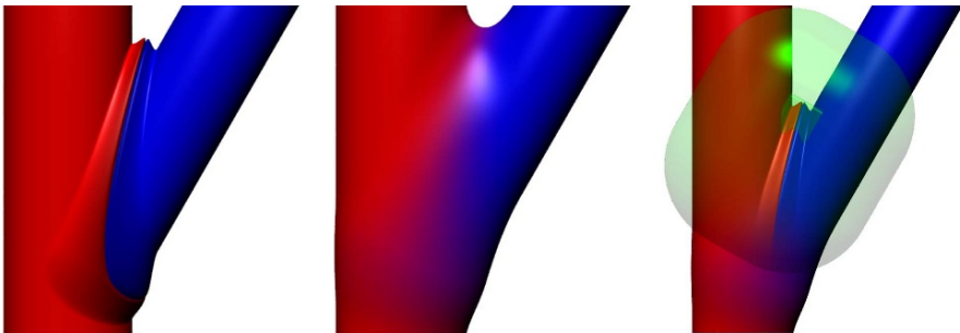
Fig. 11.7. Application of GBB to blend a lateral branch (shown in blue) to its base branch (shown in red) by interpolating between PCM (left) and summation blending (centre). The bounding field is visualised by two transparent surfaces, the inner one bounding a region where f_b = 1 and the outer one representing the zero surface f_b = 0 .
