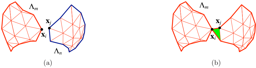
Fig. 6.20. Merging two mesh borders \Lambda_m (in thick red) and \Lambda_n (in thick blue) into a bigger border \Lambda_m (in thick red).
