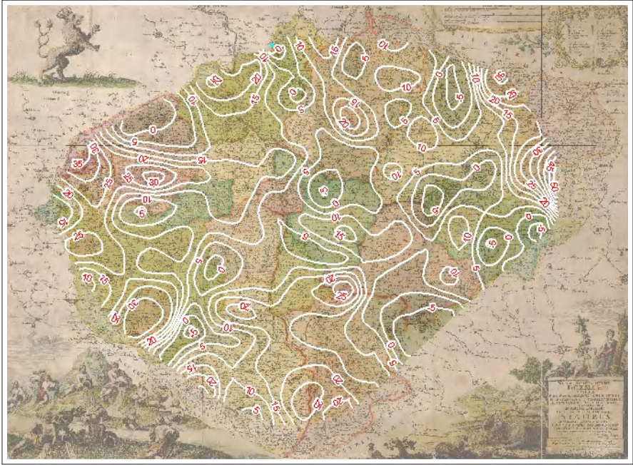
Fig. 33.7. Rotation isolines of Vogt's map generated with the step 10^\circ
