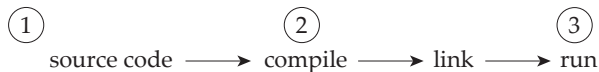
Figure 4.1: Basic tool chain from source code to running application with three points where code generation can take place (see text).
