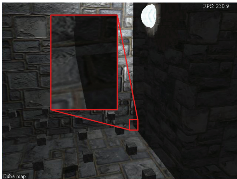
Figure 3.15. One point light and use cube shadow mapping with one 512 cube texture.
