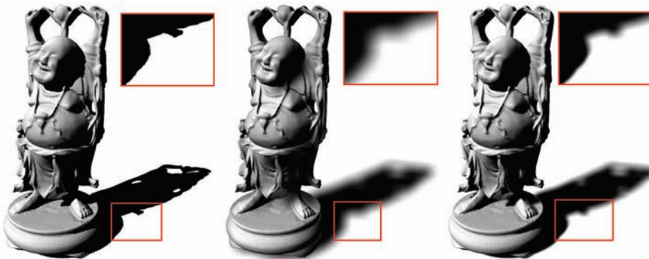
Figure 4.4. Importance of perceptually correct shadows: shadows with no penumbra (left), with uniform penumbra (middle) and with variable penumbra rendered with our method (right). Notice how the penumbra becomes sharper as the shadow approaches the occluder. Notice also the quality of self-shadows compared to uniform penumbra methods.
