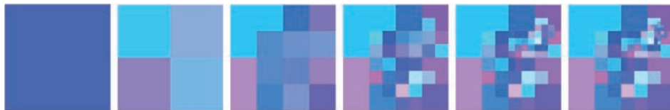
Figure 4.5. Creating the indirection texture for a camera looking over a large terrain: initializing the top level with the lowest resolution tile, we copy parent entries into the next finer level and add entries for tiles present in the cache.
