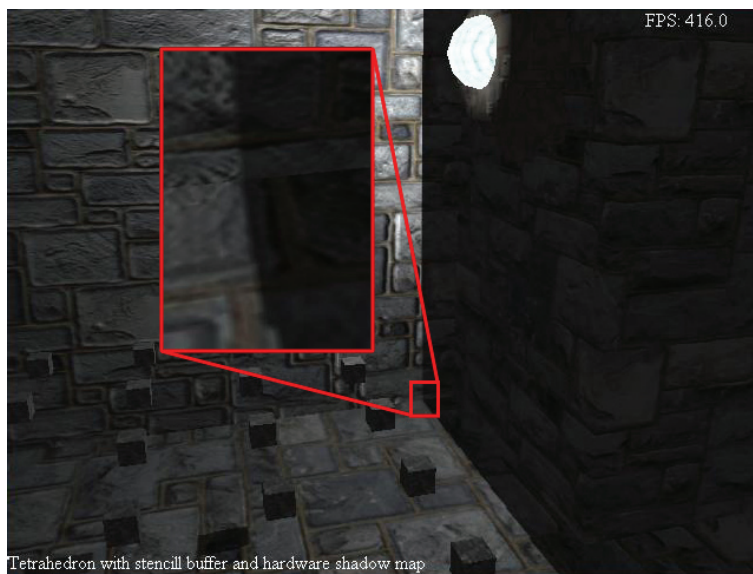
Figure 3.19. One point light and use tetrahedron shadow mapping with stencil buffer and hardware shadow mapping. The two-dimensional depth texture size is 1024 \times 1024 .
