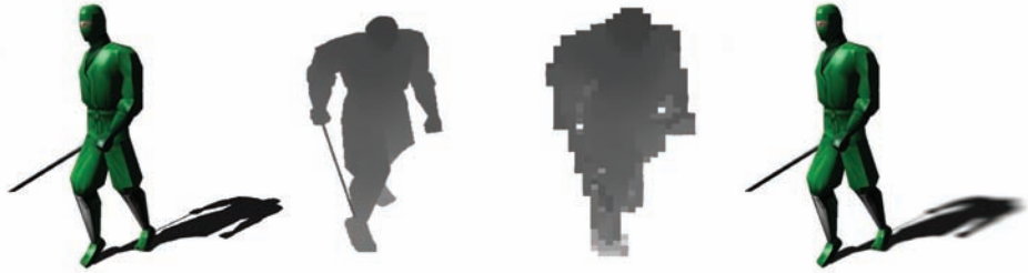
Figure 4.5. Different intermediate steps of our algorithm. From left to right: the model with hard shadows, the standard shadow map, the dilated shadow map and the final result of blurring the shadows with the anisotropic Gaussian filter.
