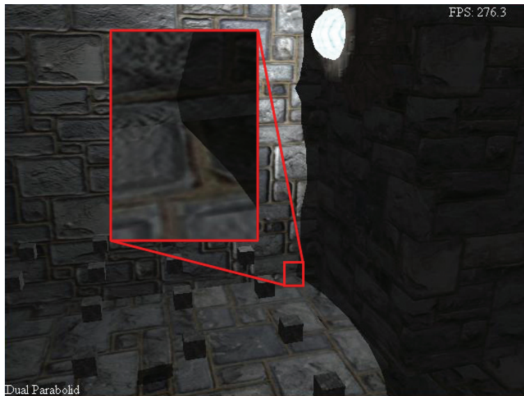
Figure 3.14. One point light and use dual-paraboloid shadow mapping with two 1024 \times 1024 two-dimensional textures.
