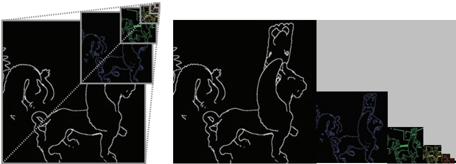
Figure 1.7. Conceptually, multiresolution rendering uses a “render-to-mipmap” approach (left). Our new stencil-based approach requires a flattened multiresolution buffer to instantiate a parallel refinement pass that sets fragment stencil bits (right).
