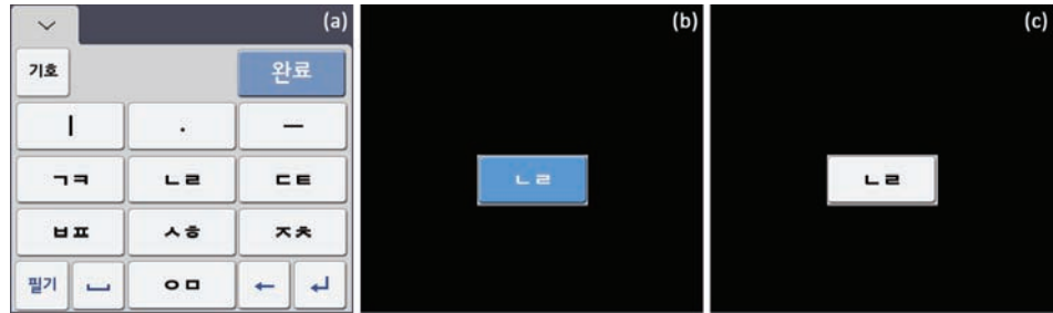
Figure 4.5. An example of partial update rendering: (a) original keypad; (b) and (c) partial update.
