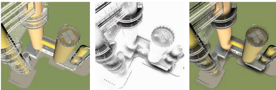
Figure 2.1. Ambient occlusion can be used to combine separately computed visibility values with the unoccluded illumination from the GPU. The left image shows the unoccluded illumination, the center image shows the ambient occlusion that darkens the cavities and contact regions only. If both are multiplied, a more realistic appearance can be obtained, as shown on the right.
