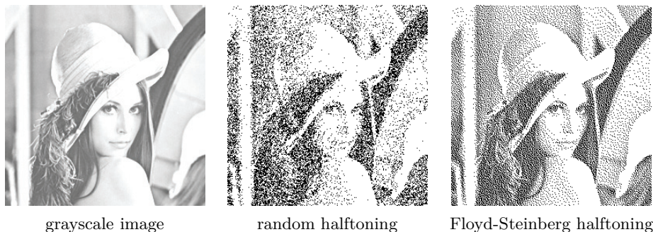
Figure 3.3. A grayscale image and its halftoned versions obtained with random halftoning and with the Floyd-Steinberg algorithm.
