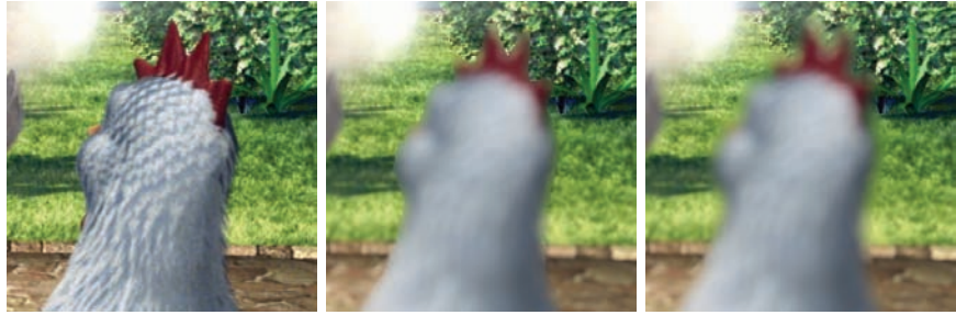
Figure 5.4. The figure shows the original rendered image, the image with defocus applied without the re-accumulation phase, and the effect of the re-accumulation step.
