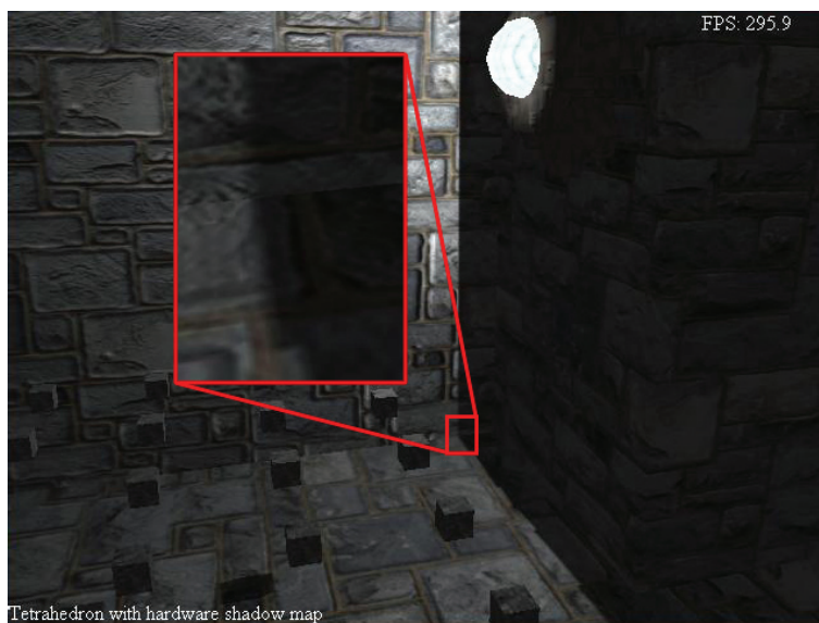
Figure 3.18. One point light and use tetrahedron shadow mapping with hardware shadow mapping. The two-dimensional depth texture size is 1024 \times 1024 .
