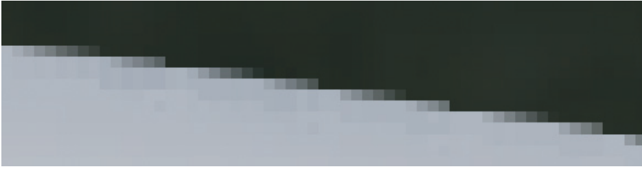
Figure 2.10. Close-up of a 2\times up-scale using edge hints. The edge is pixel-accurate at the target resolution.
