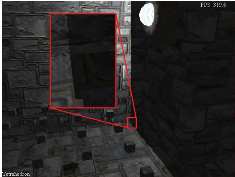
Figure 3.16. One point light and use tetrahedron shadow mapping with one 1024 \times 1024 two-dimensional texture.
