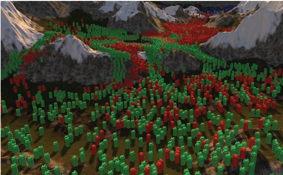
Figure 4.3. Path finding with local avoidance is implemented on the GPU using binning. Agents move from goal to goal while avoiding local obstacles and each other.
