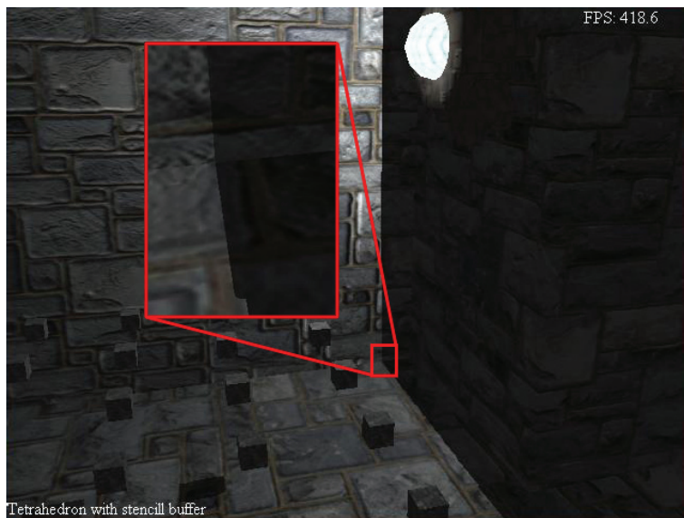
Figure 3.17. One point light and use tetrahedron shadow mapping with stencil buffer. The two-dimensional depth texture size is 1024 \times 1024 .
