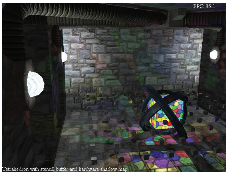
Figure 3.21. Four point lights and use tetrahedron shadow mapping with stencil buffer and hardware shadow mapping. The two-dimensional depth texture size is 1024 \times 1024 .
