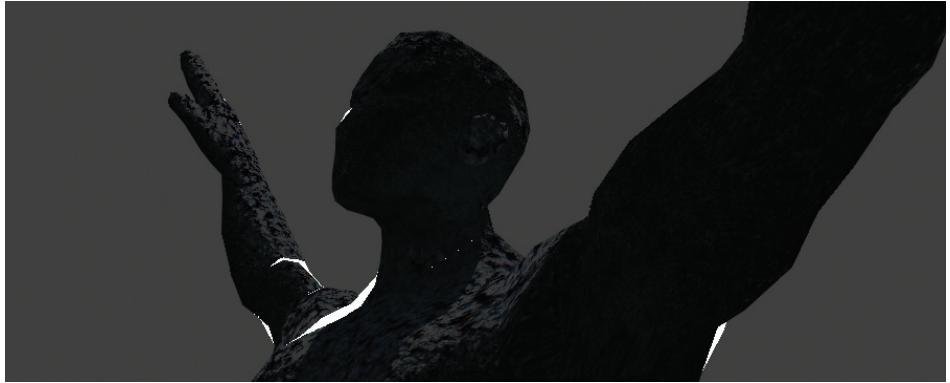
Figure 2.5. Triangles where all three vertices have passed the (low-fidelity) adjoining-back-face test have been colored white.
