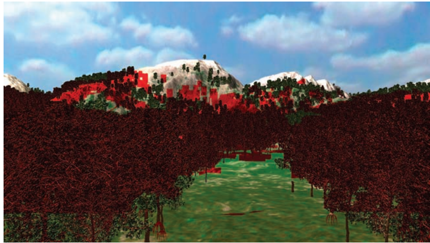
Figure 1.2. The overlapped fragments (shown in red) can be efficiently detected and discarded before shading, using Z^3 culling for increased performance. Unlike the early-Z culling approach, Z^3 culling is independent from shading operations, typically supporting programmable fragment discard and alteration of fragment depth, as well as alpha testing in this example.
