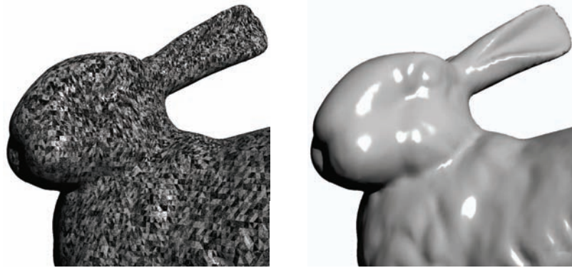
Figure 3.4. Effect of a floating-point precision error when intersecting secondary rays with primitives (left), and the image rendered after fixing this error (right). (See Listing 3.7 for details.)
