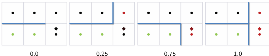
Figure 4.4. Examples of the four possible types of crossing edge and corresponding value returned by the bilinear query of the edges texture. The color of the dot at the center of each pixel represents the value of that pixel in the edges texture. The rhombuses, at a distance of 0.25 from the center of the pixel, indicate the sampling position, while their color represents the value returned by the bilinear access.
