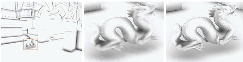
Figure 1.9. Close-up of a distant dragon in Sibenik cathedral at 1600 \times 1200 resolution: SSAO using 32 samples at 12 FPS (left close-up); TSSAO using 8–32 samples per frame at 26 FPS (right close-up).
