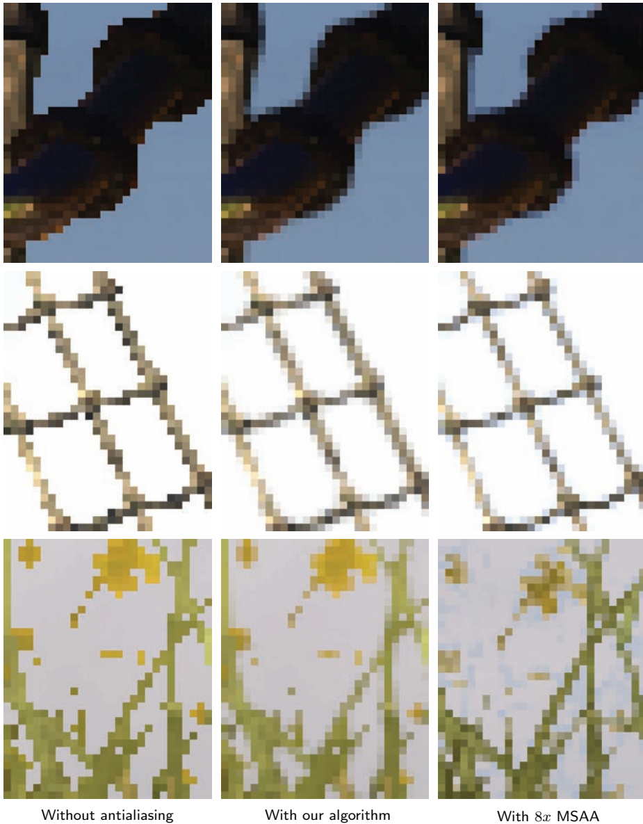
Figure 4.5. Examples of images without antialiasing, processed with our algorithm, and with 8x MSAA. Our algorithm offers similar results to those of 8x MSAA. A special case is the handling of alpha textures (bottom row). Note that in the grass shown here, alpha to coverage is used when MSAA is activated, which provides additional detail, hence the different look. As the scene is animated, there might be slight changes in appearance from one image to another. (Images from Unigine Heaven Benchmark courtesy of Unigine Corporation.)
