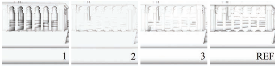
(a) If the allowed sample distance is unrestricted, shadows are cast from disconnected objects (1). If it is set equal to the sampling radius, some valid samples are not counted, resulting in overbright SSAO (2). Allowing 2 times the radius (3) is a good trade-off and closest to a ray-traced solution (REF).
