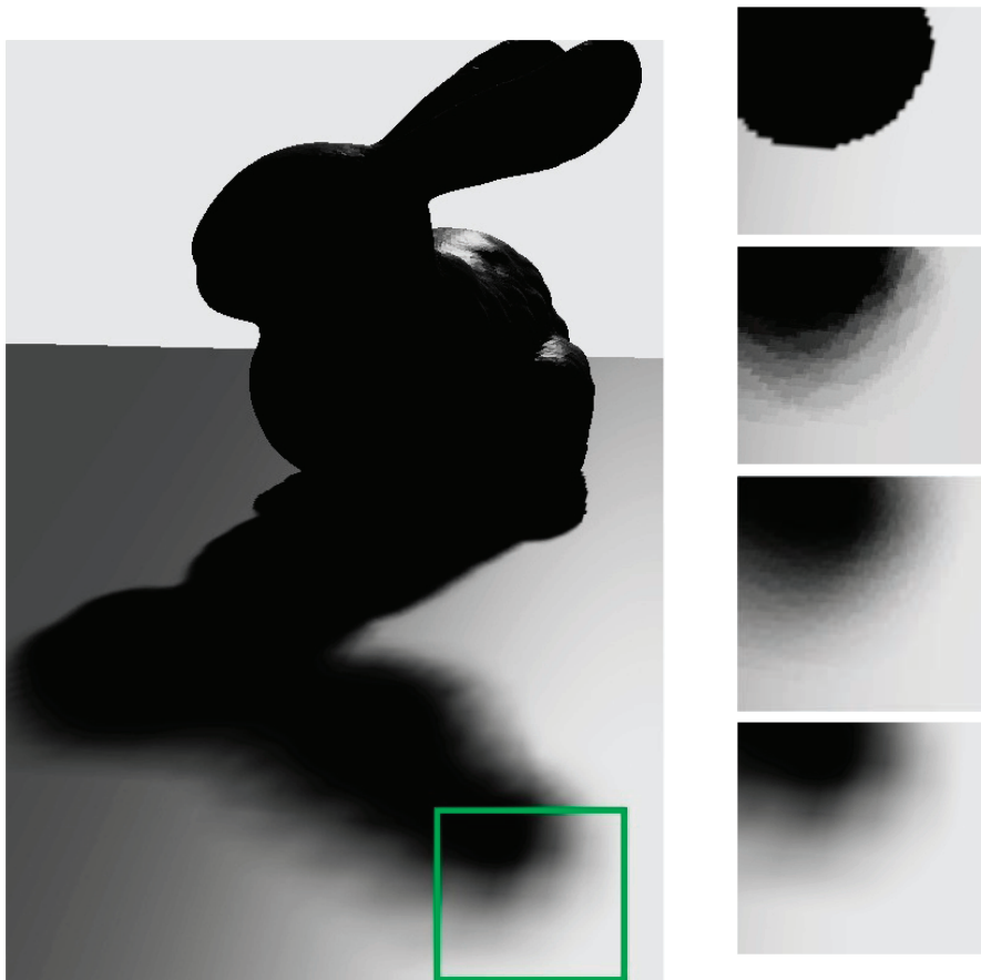
Figure 2.2. Filtering comparison. From top to bottom: bilinear PCF; 24 \times 24 PCF filter with 32 samples, frame rendering time on Radeon 4870 is 3.1 ms; 24 \times 24 PCF filter with 64 samples, 6.7 ms; 24 \times 24 MRF filter ( 3 \times 3 PCF), 3.1 ms.
