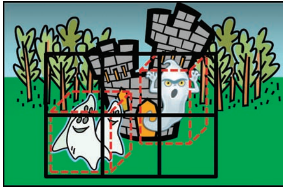
Figure 2.5. Translucent contribution to the scene is added to the render target via optimized tiling. Only tiles enclosing the bounding geometry of the translucent characters are processed. The bounding boxes of translucent geometry are transformed to screen space and the combined extents of the resulting coordinates define the minimum rectangle area that will be processed. This minimum rectangle area is covered by as many tile-sized rectangular regions as required (six in this example). Each of those regions performs fragment storing and rendering using a single pair of tile-sized head pointers and nodes buffers.
