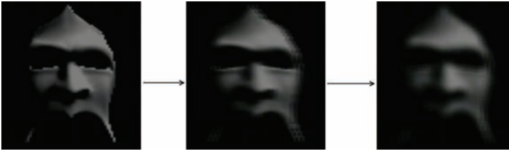
Figure 2.13. Blurring the input image in a low-resolution render target with a separated blur filter kernel.
