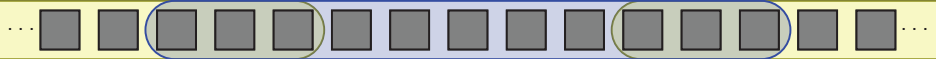
Figure 1.6. OpenCL work item for the horizontal pass (blue), with two overlapping neighbors (yellow).
