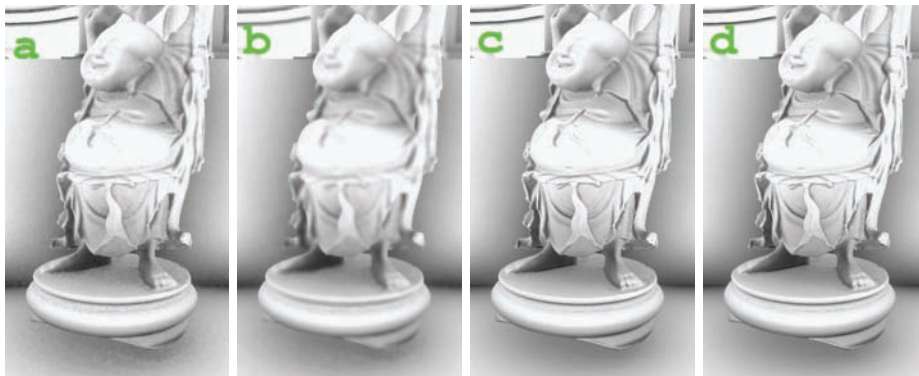
Figure 1.1. SSAO without temporal coherence (23 FPS) with 32 samples per pixel, with (a) a weak blur, (b) a strong blur. (c) TSSAO (45 FPS), using 8–32 samples per pixel (initially 32, 8 in a converged state). (d) Reference solution using 480 samples per frame (2.5 FPS). All images at 1024 \times 768 resolution and using 32-bit precision render targets. The scene has 7 M vertices and runs at 62 FPS without SSAO.
