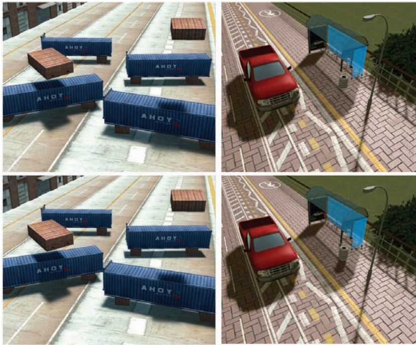
Figure 5.8. Examples of layered shadows. Light bleeding caused by incorrect computation of the distance between the occluder and the receiver (top). Layered shadow maps can reduce occluder problems (bottom).
