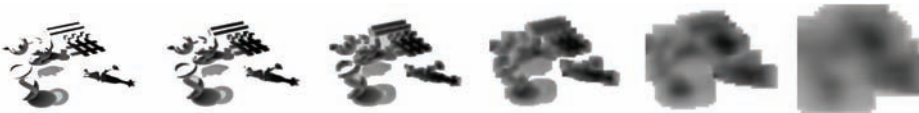
Figure 5.3. Mipmap levels obtained by flood filling. The flood fill propagates information from hard shadows to outer regions.
