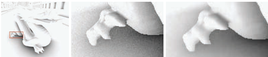
Figure 1.6. Rotating dragon, closeups of the marked region are shown. TSSAO without filter (middle) and with our filter (right). Note that the filter is applied only in the noisy regions, while the rest stays crisp.
