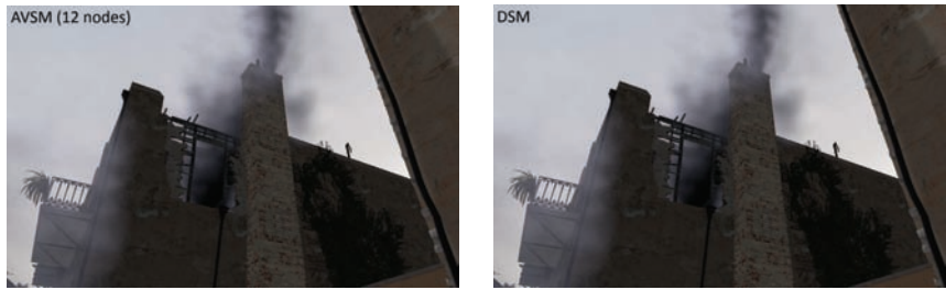
Figure 3.3. A comparison of smoke added to a scene from a recent game title with AVSM with 12 nodes (left) and deep shadow maps (right). Rendering the complete frame takes approximately 32 ms, with AVSM generation and lookups consuming approximately 11 ms of that time. AVSM is 1–2 orders of magnitude faster than a GPU implementation of deep shadow maps and the uncompressed algorithm, yet produce a nearly identical result. (Thanks to Valve Corporation for the game scene.)
