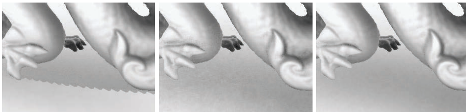
Figure 1.5. Rotating dragon model using different values for smooth invalidation factor S . (left) S = 0 (i.e., no invalidation), (middle) S = 100 , (right) S = 15 . Note that no invalidation causes a wrong shadow (left), while a too high value causes unwanted noise in the shadow (middle).
