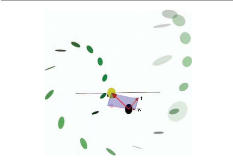
Figure 13.4: The computation of the screw corresponding to a rotor R followed by a translation over \mathbf{t} . The rotor plane and angle are indicated by the blue disk. The translation \mathbf{w} along the screw axis is the rejection of \mathbf{t} by the rotation plane. The location vector \mathbf{v} of the axis is found as the unique vector in the rotation plane whose chord under rotation is parallel to \mathbf{w} - \mathbf{t} (indicated by a thin blue line). The resulting screw motion around the axis (in black) is shown applied to a tangent bivector (in fading shades of green).
