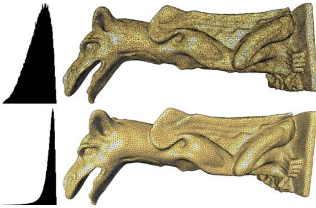
Figure 14: Gargoyle: a comparison with [Cutler et al. 2004] further demonstrates the excellent results of a variational approach. Our distribution in terms of radius ratios (one of the fairest measures [Shewchuk 2002a]) is far superior to a standard optimization technique (mesh courtesy B. Cutler).
