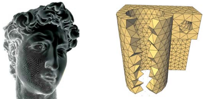
Figure 1: Typical 2D and 3D meshes: although the David's head appears smooth, its surface is made of a triangle mesh; tetrahedral meshes (such as this mechanical part, with a cutaway view) are some typical examples of irregular meshes on which faithful computations need to be performed. David's head mesh is courtesy of Marc Levoy, Stanford.
