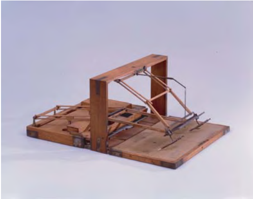
Figure 1.3. A pantograph. Joint x is pinned. The movement of joint y is duplicated and doubled by point z .
