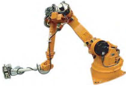
Figure 1.2. A six-axis robot arm. [By permission, Forward Thompson Ltd.]
