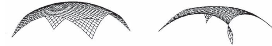
Fig. 6. Bicubic surface patch with line of vanishing Gaussian curvature (left). Orthotomic analysis (right).
