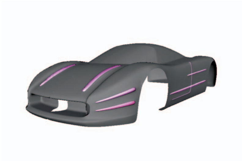
Fig. 17. Insertion of different Sweep-like features on a car model.
