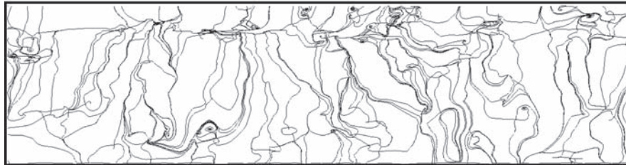
Fig. 5. Topological skeleton of the skin friction data set.
