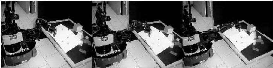
Fig. 13.20. Image sequence of a linear-path motion
