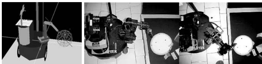
Fig. 13.22. (a) ( left ) Simulation of the motion over a sphere. (b) and (c) ( right ) Two of the images in the sequence of the real experiment
