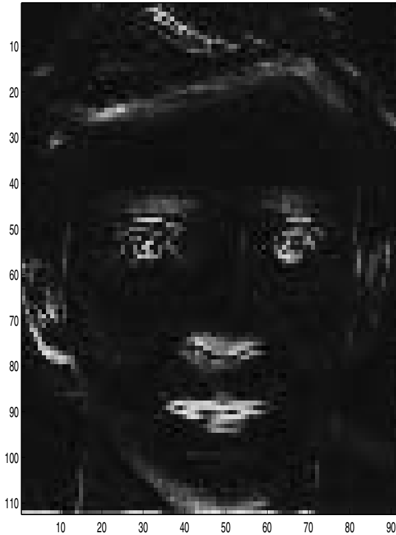
Fig. 2.5. The reconstruction of basic face features from extrema by summing values at corresponding grid points at different scales. The extrema representation is approximately 50 times more compressed than the corresponding GIF image.
