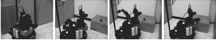
Fig. 13.12. Full calibration: after the laser and the binocular systems are calibrated, the robot can navigate and reach objects in 3-D accurately
