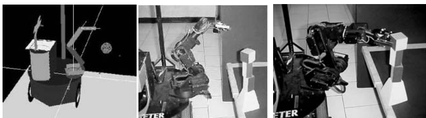
Fig. 13.23. (a) Algorithm simulation showing the sphere containing the cube. (b) Image of the object we wish to grasp with the robotic arm. (c) The robot “Geometer” grasping a wooden cube
