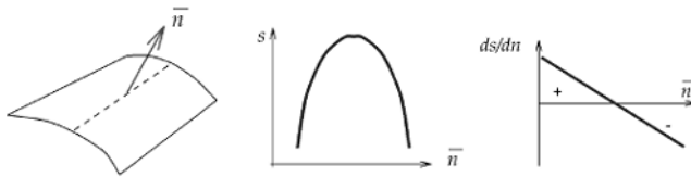
Fig. 16.4. Dense surface extraction in 3-D: (Left) Elementary surface patch with normal \mathbf{n} . (Center) 3-D surface saliency along normal direction (Right) First derivative of surface saliency along normal direction
