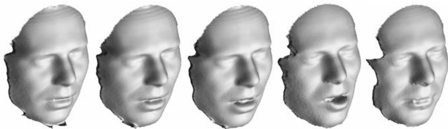
Figure 12.4. An example of a three-dimensional video acquired with a coded light range scanner at 3 frames per second. Photometric information (texture) is not shown.
