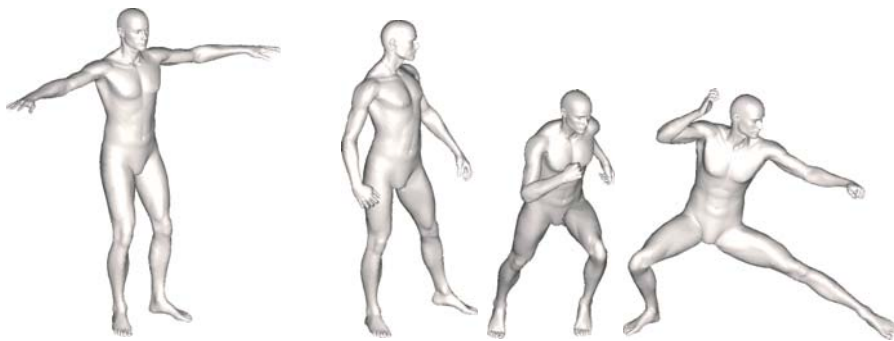
Figure 10.4. Symmetric or not? Extrinsically symmetric shape is also intrinsically symmetric (left), however, isometries of the shape are intrinsically symmetric but extrinsically asymmetric (three rightmost shapes).
