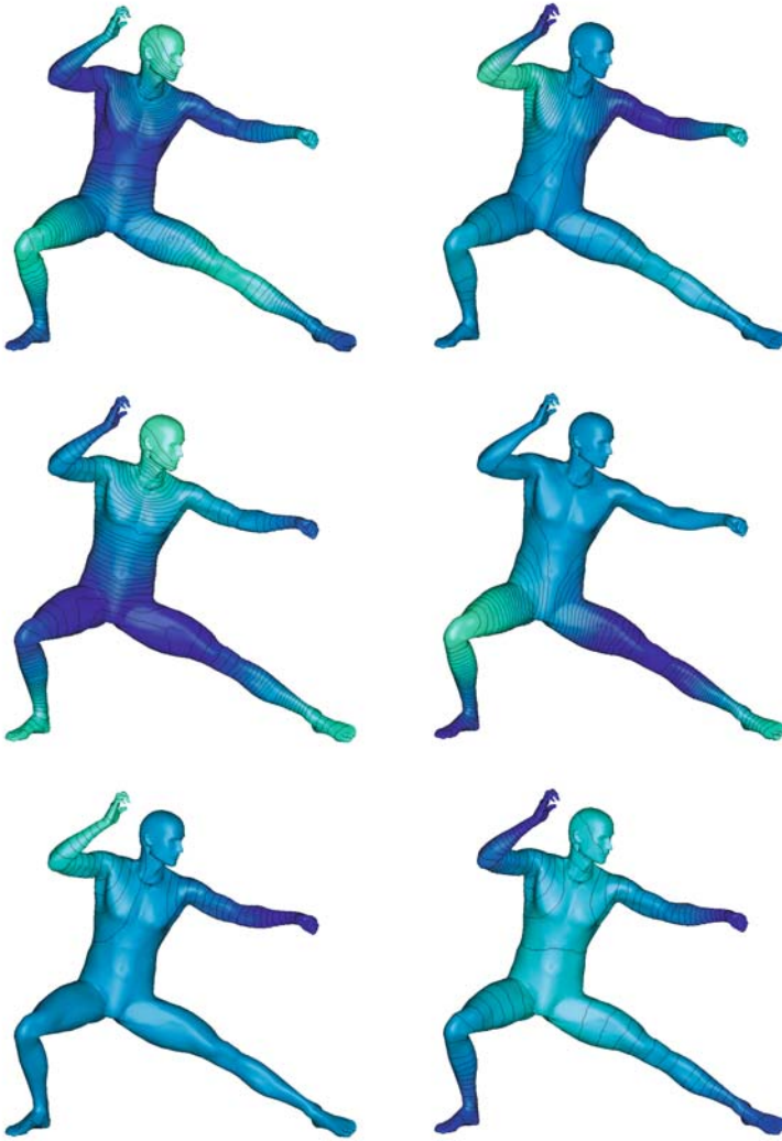
Figure 8.3. The first non-trivial eigenfunctions of the Laplace-Beltrami operator of a human shape. Colors and contours visualize the values of the eigenfunctions at each point of the shape.
