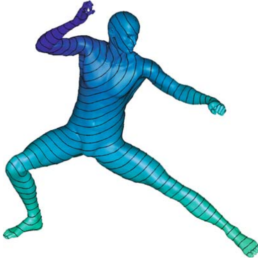
Figure 4.7. Distance map measured on a triangular mesh. Equidistant contours from the source located at the right hand are shown.
