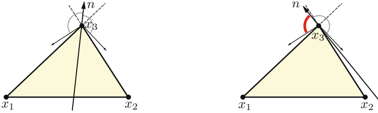
Figure 4.5. The monotonicity condition QV^T n < 0 requires the wavefront propagation direction n to form obtuse angles with the normals to the triangle edges (x_3, x_1) and (x_3, x_2) . Geometrically, this can be interpreted as demanding n to lie within the triangle (left). Right: update direction violating the monotonicity condition lies outside the triangle.
