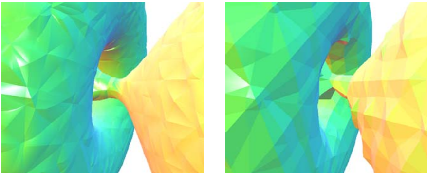
Fig. 8. Closeup view of hydrogen atom dataset rendered with quadratic patches( left ). As in Fig. 5, the isosurface extracted using linear elements( right ) shows the resolution of the underlying tetrahedral grid. Isovalue = 9.4, Error = 0.566
