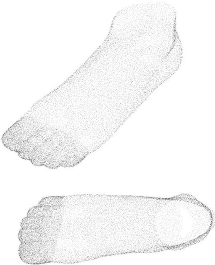
Fig. 16. This data is courtesy of Geomagic. The data is noisy, the sampling density is not uniform and there are regions of missing data near the heel, the balls and the ankle
