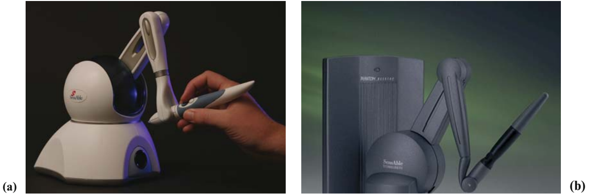
Figure 10.5 Exemplar desktop haptic interaction tools (force feedback). In (a) the PHANTOM Omni™ 6-DOF device and in (b) the PHANTOM Desktop™ which also offers 6-DOF. For technical details see Table 10.1. (Images supplied by, and reproduced with the permission of SensAble Technologies Inc.®.)
