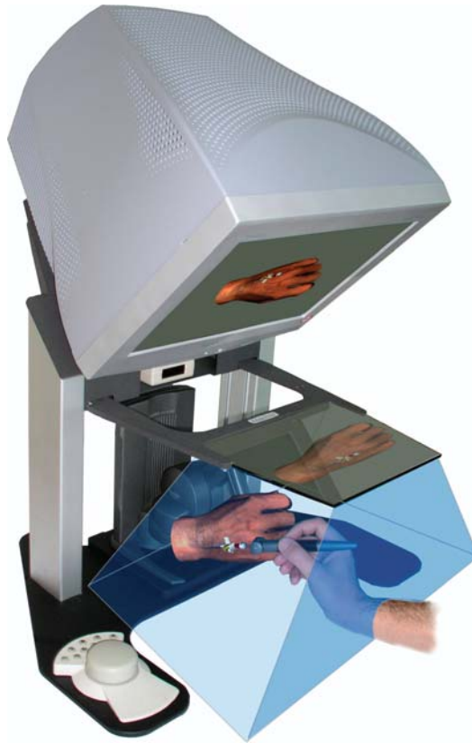
Figure 9.7 A commercial display system produced by Reachin Technologies. 6 The basic principle of operation of this system is based on the Pepper's (Dircks') Ghost illusion which dates back to the 1860s. As can be seen, from this artist's rendition, the reflected image appears to reside behind the glass plate. Thus the user's hand and interaction tool appear to coexist within the same virtual image space. This system employs a 19 inch CRT based display (1024 by 768 pixels) that is refreshed at 120 Hz (giving a 60 Hz refresh frequency for each eye). The stereo viewing glasses are of the shutter type and are connected by means of a wireless link. (Image kindly supplied by and reproduced by permission of Reachin Technologies AB.)
