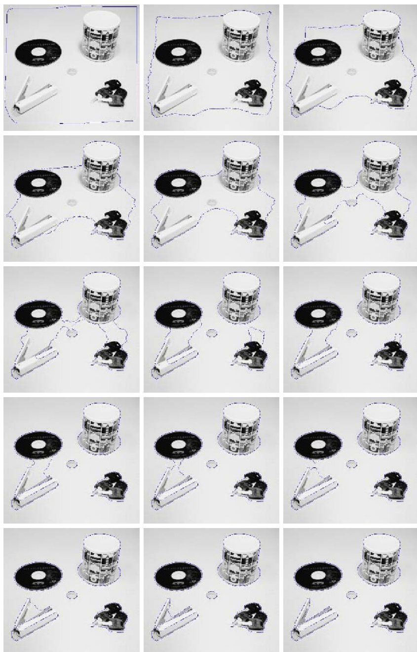
Figure 4.13. Segmentation of the “objects” image using the geodesic active contour model (4.55). From top left to bottom right, different iterations (solution as time evolves) are displayed. Initialized by the boundaries of the images, the curve is shrinking and splitting until it isolates each object.
