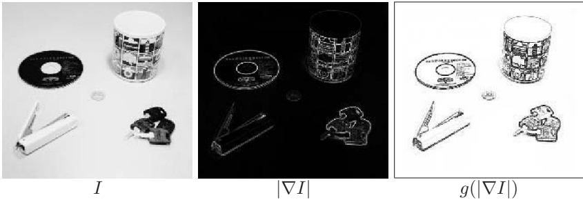
Figure 4.8. Example of edge detector function. g(s) = \frac{1}{1+s^2} has been chosen for the right-hand side image. Noise is reduced and contours are enhanced. Also note the inversion of colors due to the function g .
