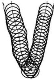
(a) Local overcut (gouge)
