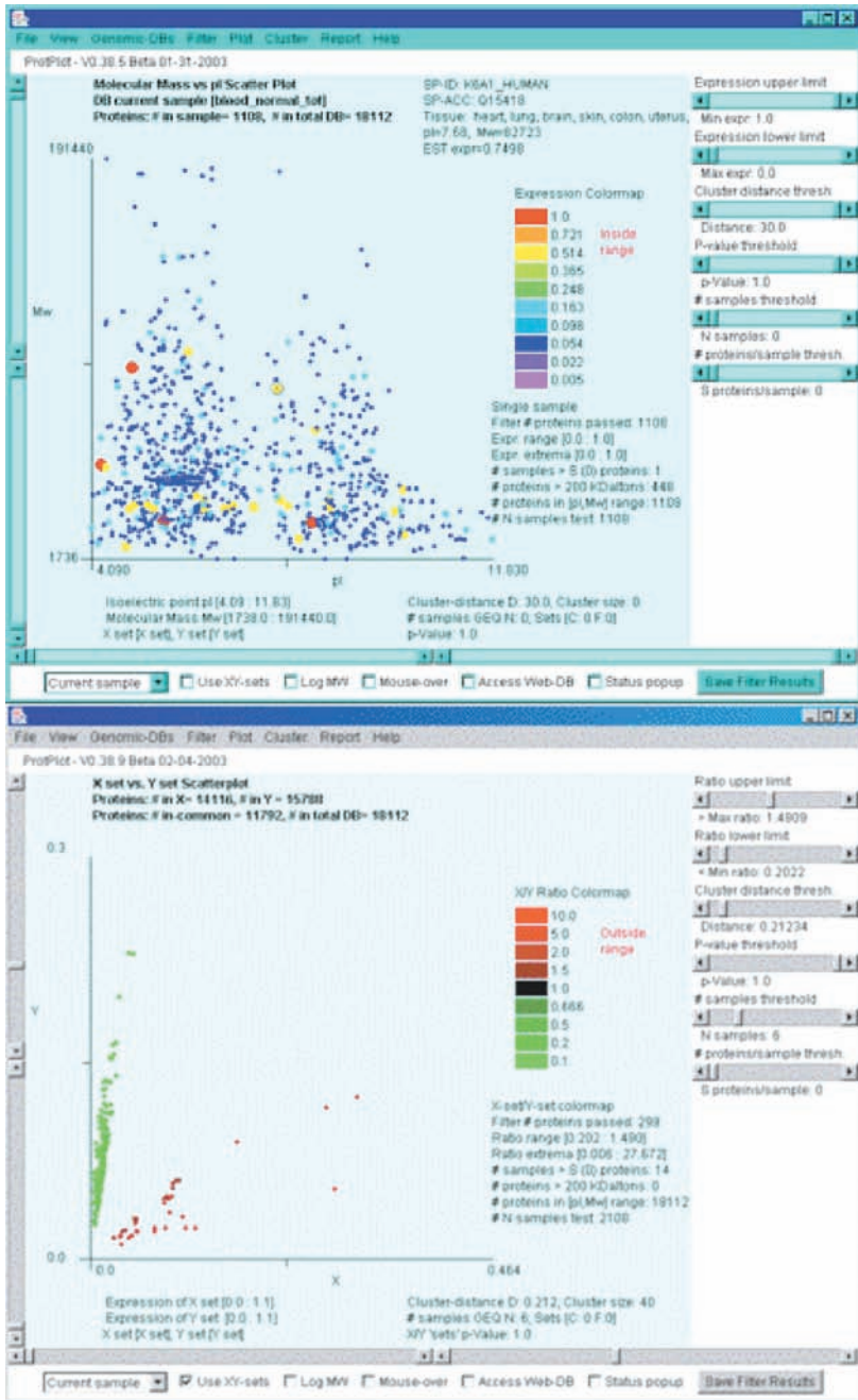
FIGURE 6.15 Snapshot of scatterplots from one sample in ProtPlot (top). It is also possible to create (bottom) an (X vs. Y) scatterplot or (mean X set vs. mean Y set) scatterplot when the corresponding ratio display mode is set. The following window shows the (mean X set vs. mean Y set) scatterplot.
