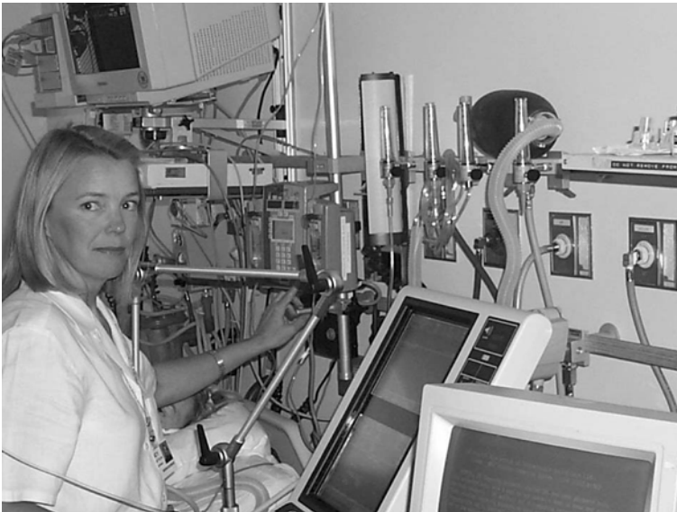
Figure 17.1. A nurse at a patient's ICU bedside. Above the nurse's head is the bedside monitor which measure and displays key physiological data, above her left hand is an IV pump connected to a Medical Information Bus (MIB), to her right are two screens of a patient ventilator and to the far right is a bedside computer terminal used for data entry and data review. ( Source: Courtesy of Dr. Reed M. Gardner)
