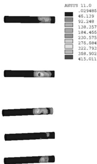
Fig. 4 Equivalent stresses in the bone screws calculated for the applied loading F = 800 N
