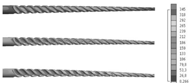
Fig. 5 Distribution of reduced stresses in X39Cr13 steel drill's working section: a) \varphi = 1^\circ , b) \varphi = 2^\circ , c) \varphi = 1^\circ
