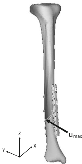
Fig. 6 Equivalent displacements in the OZ axis calculated for the applied loading F = 800 \text{ N}
