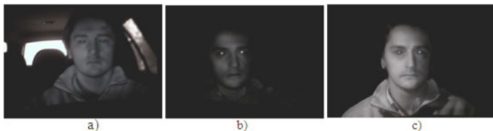
Fig. 4 Image of driver's face by: a) day, b) night, c) night with side illumination
