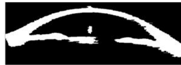
Fig. 9 Binary image after the hole-filling operation
