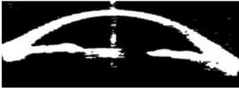
Fig. 8 Binary image obtained by binarization of the original image with a threshold of 90% of maximum value
