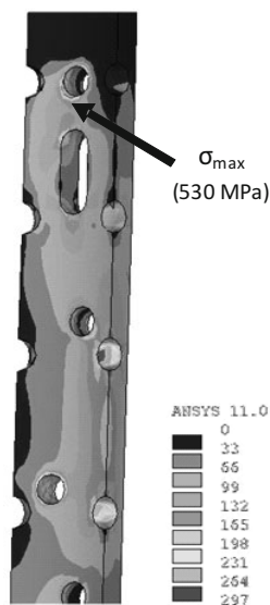
Fig. 5 Equivalent stresses in the plate calculated for the applied loading F = 800 N
